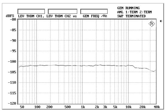
Fig.5 THD+N vs. input frequency (@-1dB)
