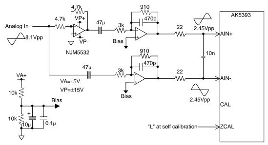
Figure 1. Full-differential input buffer circuit example
