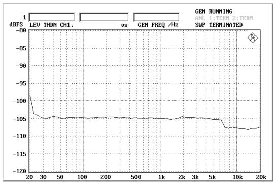
Fig.5 THD+N vs. input frequency (@-1dB)
