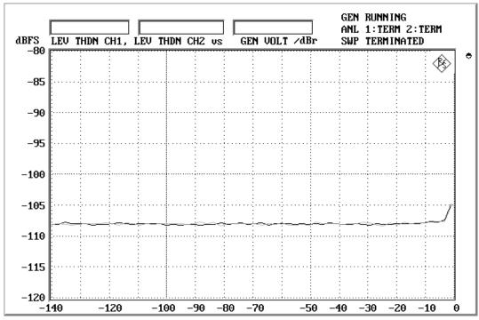
Fig.6 THD+N vs. input level ( @ frequency = 1kHz)
