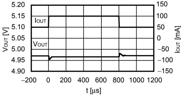
$V_{IN} = 5.5\text{ V}$ ,  $C_{OUT} = 4.7\ \mu\text{F}$ ,  $C_{IN} = 4.7\ \mu\text{F}$ ,  $I_{OUT} = 100 \leftrightarrow 500\text{ mA}$
