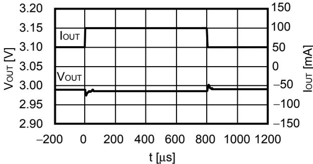
$V_{IN} = 4.0\text{ V}$ ,  $C_{OUT} = 4.7\ \mu\text{F}$ ,  $C_{IN} = 4.7\ \mu\text{F}$ ,  $I_{OUT} = 100 \leftrightarrow 500\text{ mA}$
