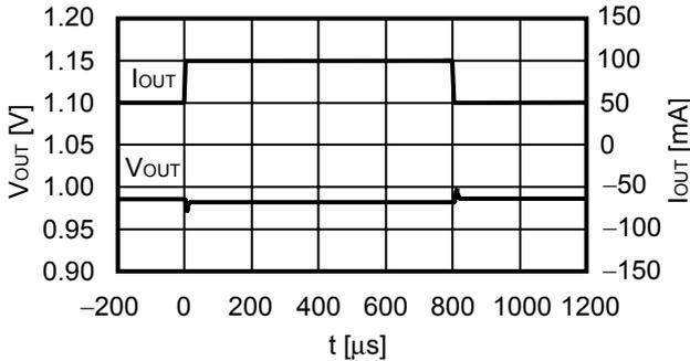
$V_{IN} = 2.0\text{ V}$ ,  $C_{OUT} = 4.7\ \mu\text{F}$ ,  $C_{IN} = 4.7\ \mu\text{F}$ ,  $I_{OUT} = 100 \leftrightarrow 500\text{ mA}$
