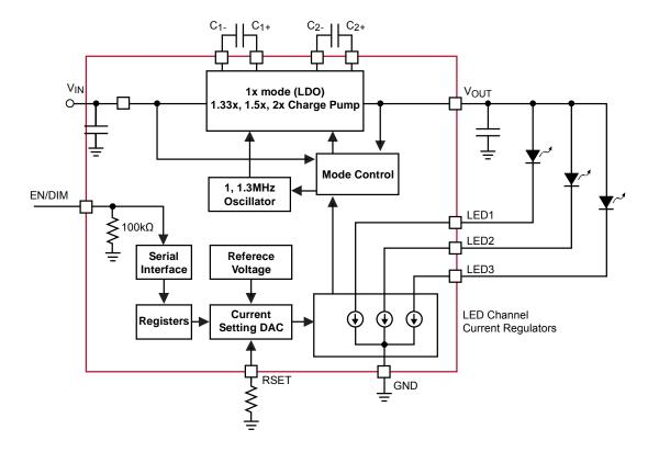
Figure 2. CAT3643 Functional Block Diagram
