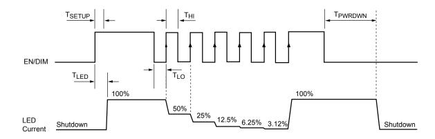
Figure 1. EN/DIM Digital Dimming Timing Diagram
