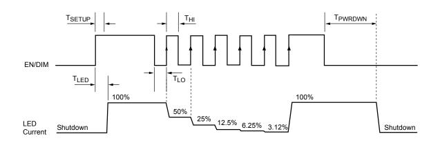
Figure 3. EN/DIM Digital Dimming Timing Diagram
