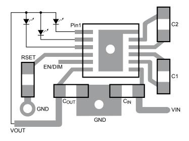
Figure 5. TDFN-12 Recommended Layout
