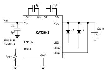
Figure 4. Application with 2 LEDs
