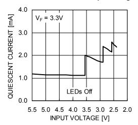
LED Current Change vs. Input Voltage
