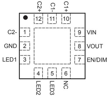
The CAT3643 is offered in three different packages. The 12-lead TDFN 3mm x 3mm with a max height of 0.8mm is pin-compatible to the Catalyst CAT3603 LED driver. The 12-lead XQFN provides the smallest
