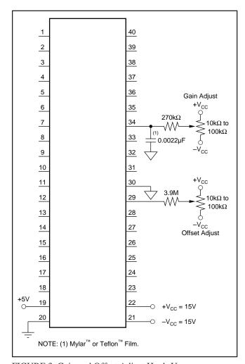
FIGURE 3. Gain and Offset Adjust Hook-Up.
