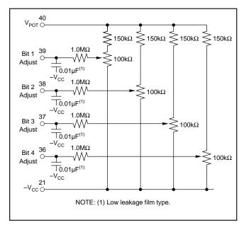
FIGURE 12. Differential Linearity Adjustment Circuit for the 4MSBs.
