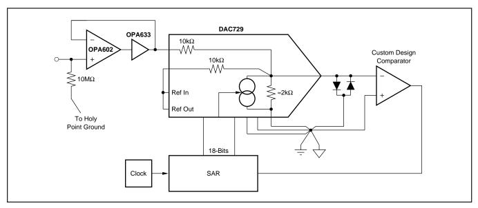
FIGURE 15. Block Diagram of an 18-Bit Resolution  $\pm 10V_{_{\rm I\!N}}$  ADC.
