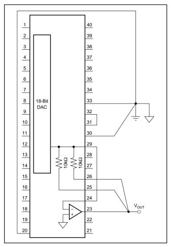
FIGURE 13. 0 to 10V FSR.
