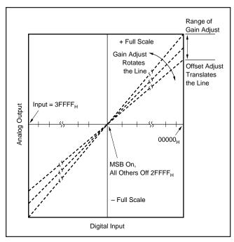
FIGURE 8. Effect of  $V_{\text{REF}}$  Adjust on a COB Connected DAC729.
