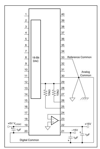
FIGURE 2. Ground Connections and Supply Bypass.
