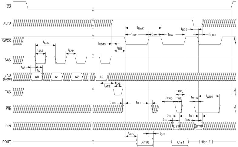
Note: Out of ten bits from A0 to A9, only the eight bits from A0 to A7 are effective. Fix A8 and A9 to "L".
