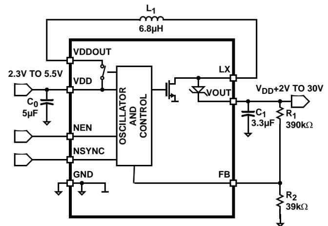
NOTE:  $V_{OUT} = (390k + 39k)/39k * 1.15V = 12.65V$
