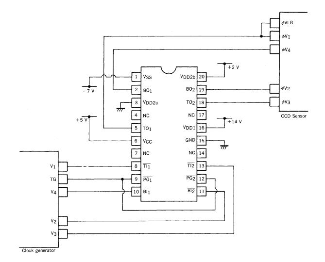
Note 1. Turn on the power  $V_{DD1}$  before  $V_{CC}$  and  $V_{DD2}$ 2. PG<sub>1</sub> (terminal 9) and PG<sub>2</sub> (terminal 12) are able to input both common signal and different signal.
