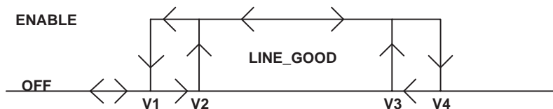
Figure 2. Line UVLO and OVLO Operation
