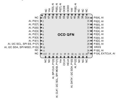
Figure 4. CY8C20000 48-Pin OCD PSoC Device
