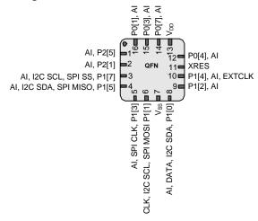
Table 5. Pin Definitions - CY8C20234 16-Pin (QFN no e-pad)
