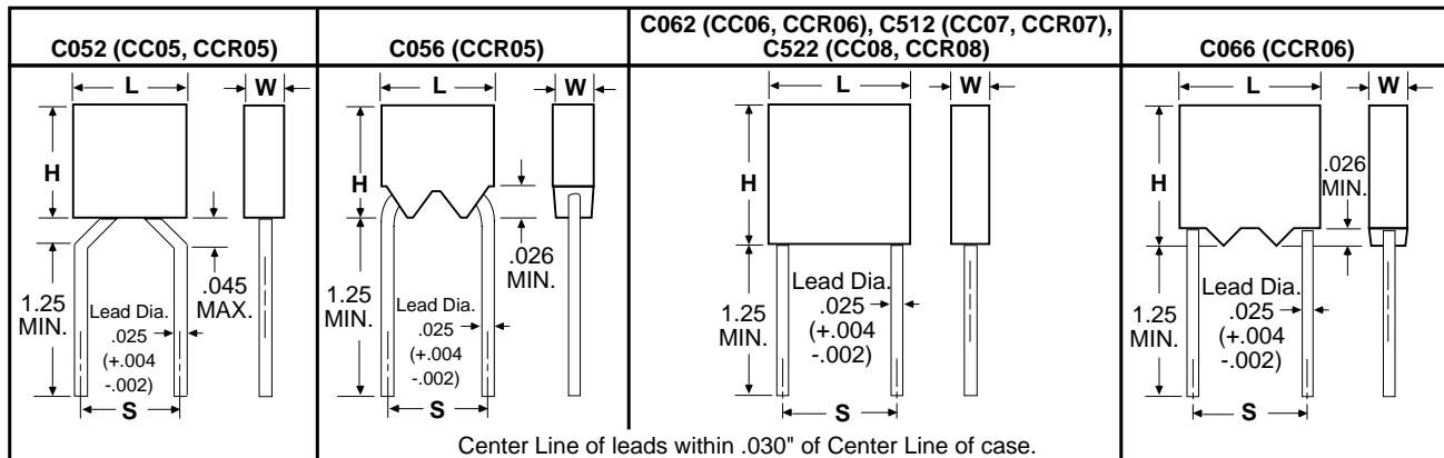
\* Leads are .625 minimum when tape and reel packaged
