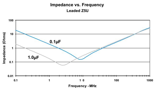
Figure 12. Impedance vs Frequency
