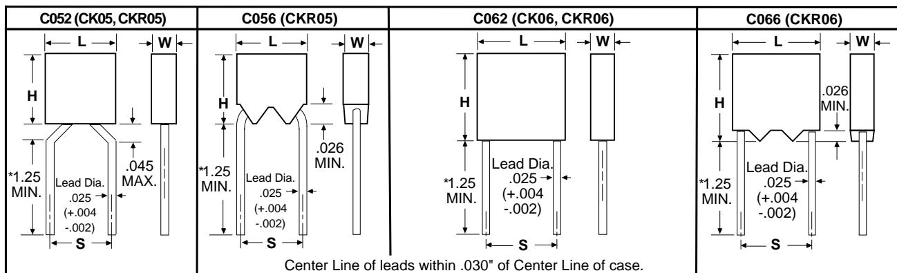
\* Leads are .625 minimum when tape and reel packaged.
