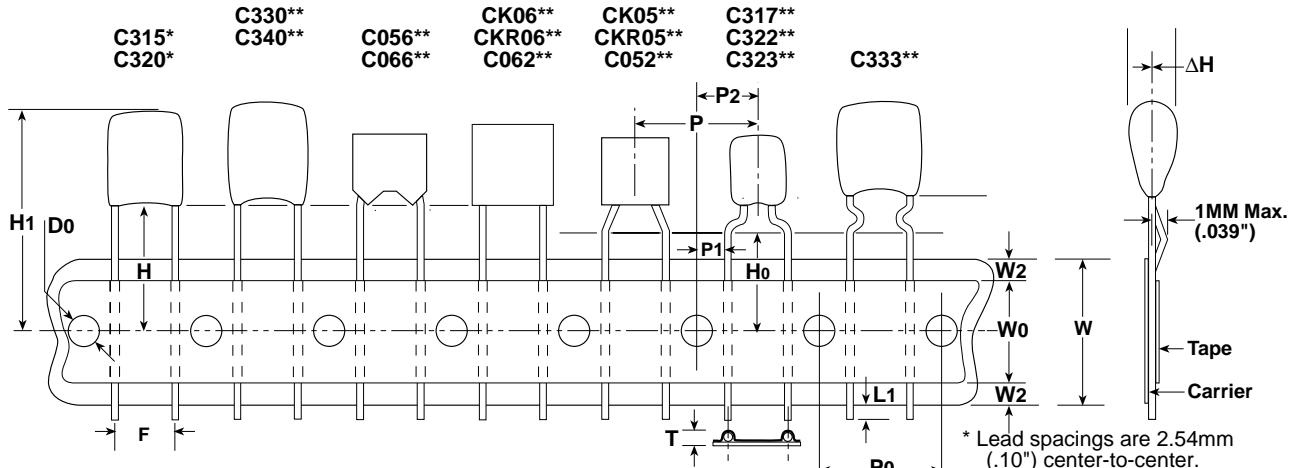
**Figure 2: Lead Tape Configuration (See Table Below)**
