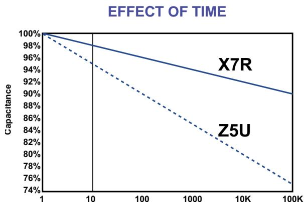
Figure 13. Typical Aging Rates for X7R & Z5U
