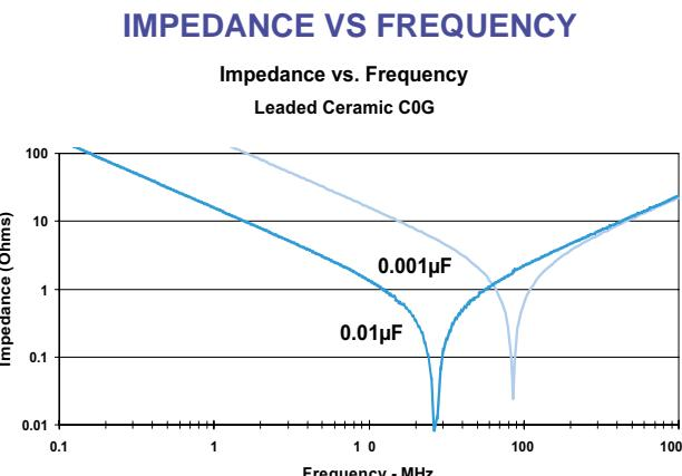
Figure 10. Impedance vs Frequency
