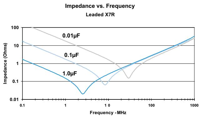
Figure 11. Impedance vs Frequency
