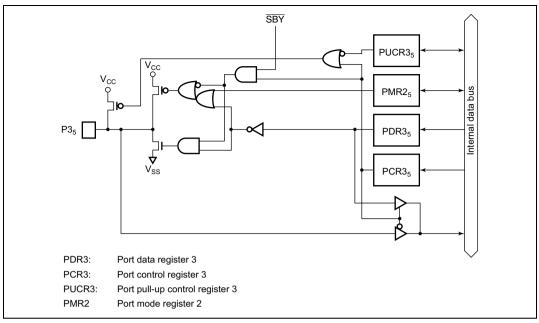
Figure C.2(b) Port 3 Block Diagram (Pin P3<sub>5</sub>)
