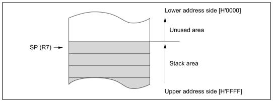
Figure 2.2 Stack Pointer
