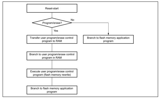
Figure 6.9 Programming/Erasing Flowchart Example in User Program Mode
