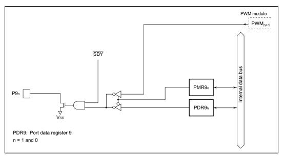
Figure C.8(a) Port 9 Block Diagram (Pins P9<sub>1</sub> and P9<sub>0</sub>)
