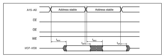
Figure 6.15 CE and OE Enable State Read Timing Waveforms
