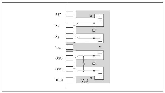
Figure 4.12 Example of Crystal and Ceramic Oscillator Element Arrangement
