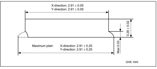
Figure G.3 Chip Sectional Figure of the HCD64338024S, HCD64338023S, HCD64338022S, HCD64338021S, and HCD64338020S
