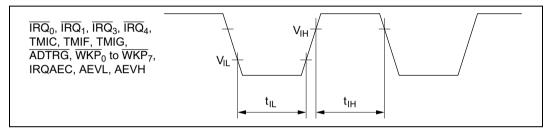
Figure 16.3 Input Timing
