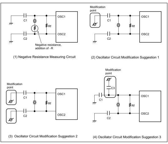
Figure 4.13 Negative Resistance Measurement and Circuit Modification Suggestions
