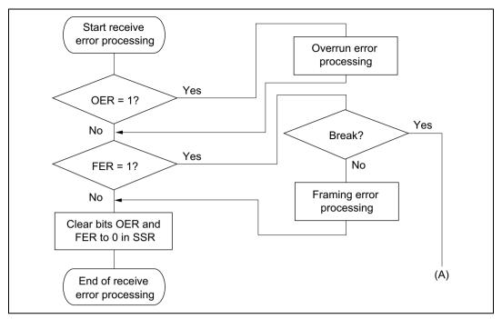
Figure 10.19 Example of Multiprocessor Data Reception Flowchart (cont)
