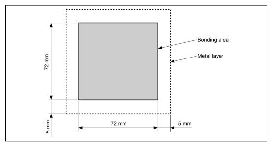
Figure H.1 Bonding Pad Form
