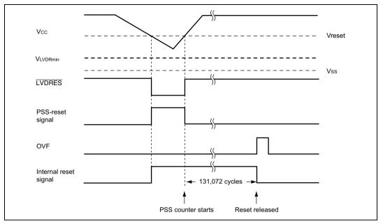
Figure 14.3 Operational Timing of LVDR Circuit
