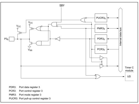
Figure C.2(e) Port 3 Block Diagram (Pin P3<sub>0</sub>)
