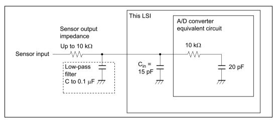
Figure 12.8 Analog Input Circuit Example
