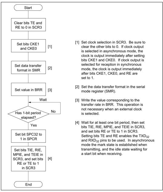
Figure 10.5 Example of SCI3 Initialization Flowchart
