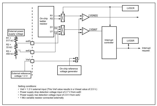
Figure 14.6 shows a usage example for the LVD function employing pins Vref, extD, and extU.
