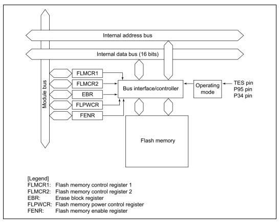
Figure 6.7 Block Diagram of Flash Memory
