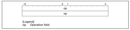
Figure 2.10 Block Data Transfer Instruction Code
