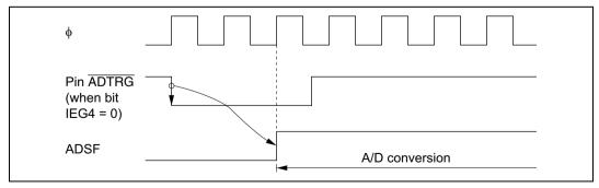
Figure 12.2 External Trigger Input Timing
