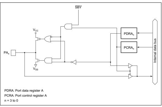
Figure C.9 Port A Block Diagram
