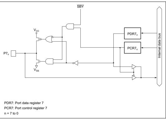
Figure C.6 Port 7 Block Diagram
