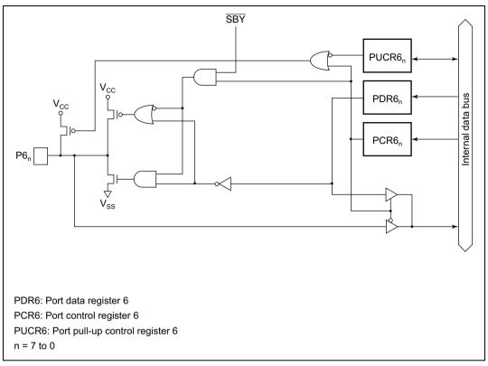
Figure C.5 Port 6 Block Diagram
