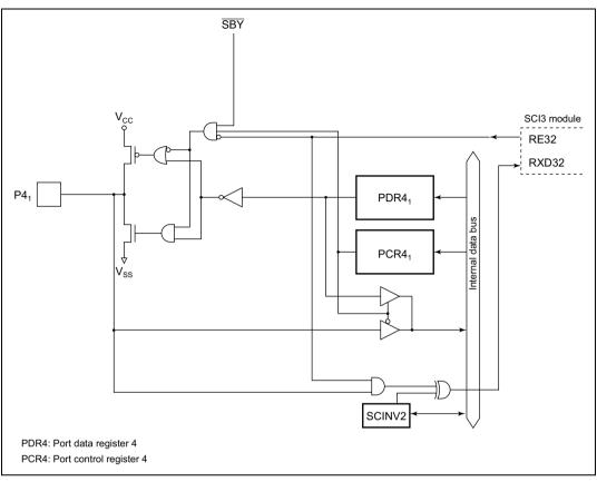
Figure C.3(c) Port 4 Block Diagram (Pin P4<sub>1</sub>)
