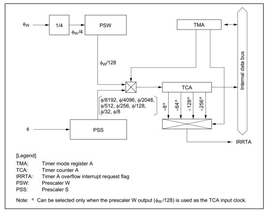
Figure 9.1 Block Diagram of Timer A
