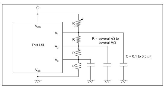
Figure 13.9 Connection of External Split-Resistance
