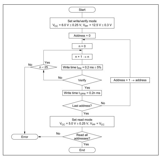
Figure 6.4 High-Speed, High-Reliability Programming Flowchart
