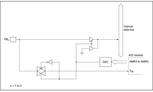
Figure C.10(a) Port B Block Diagram
