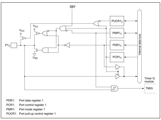
Figure C.1(c) Port 1 Block Diagram (Pin P1<sub>3</sub>)
