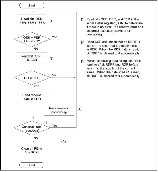
Figure 10.8 Example of Data Reception Flowchart (Asynchronous Mode)
