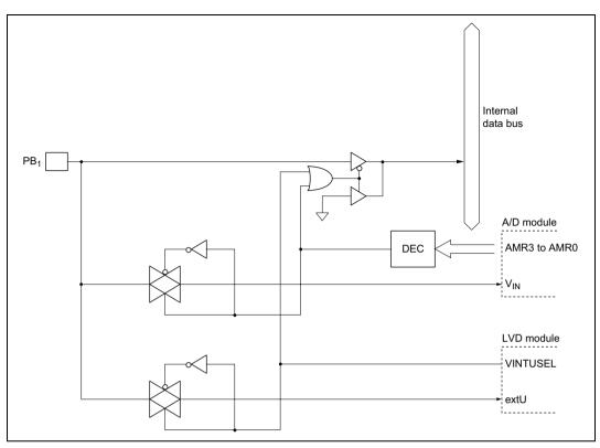
Figure C.10(c) Port B Block Diagram (Pin PB<sub>1</sub>, H8/38124 Group only)
