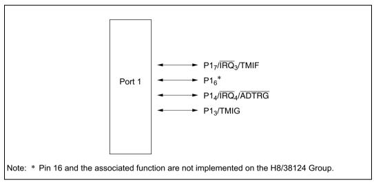
Figure 8.1 Port 1 Pin Configuration
