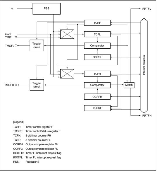
Figure 9.3 Block Diagram of Timer F
