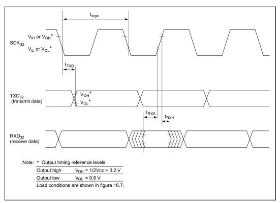
Figure 16.5 SCI3 Synchronous Mode Input/Output Timing
