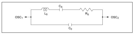
Figure 4.4 Equivalent Circuit of Crystal Oscillator
