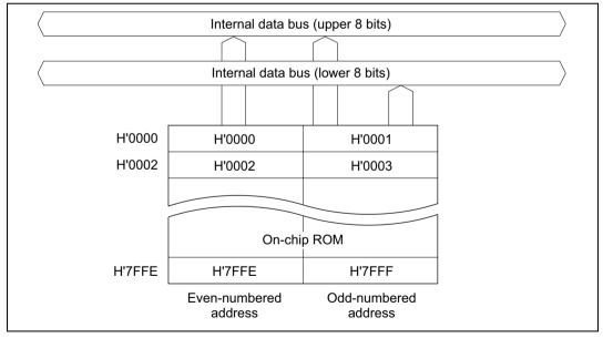
Figure 6.1 ROM Block Diagram (H8/38024)
