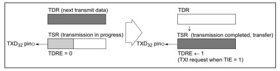
Figure 10.2(b) TDRE Setting and TXI Interrupt
