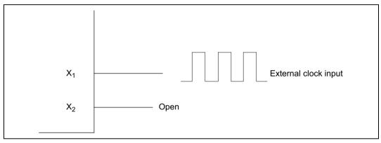
Figure 4.11 Pin Connection when Inputting External Clock
