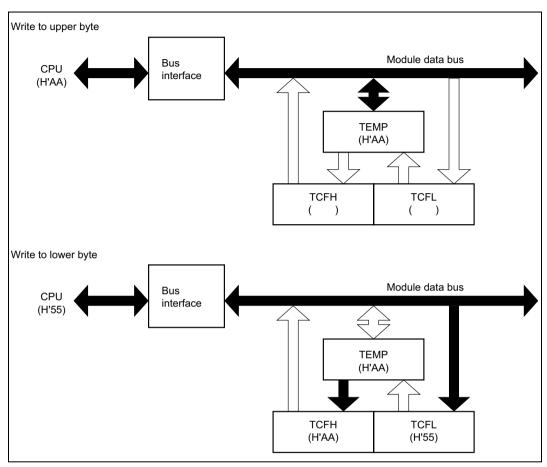
Figure 9.4 Write Access to TCF (CPU  $\rightarrow$  TCF)
