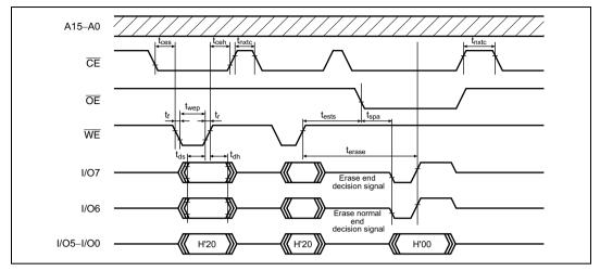
Figure 6.18 Auto-Erase Mode Timing Waveforms
