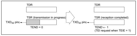
Figure 10.2(c) TEND Setting and TEI Interrupt
