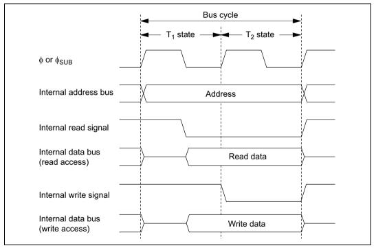
Figure 2.11 On-Chip Memory Access Cycle
