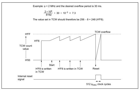
Figure 9.18 Typical Watchdog Timer Operations (Example)
