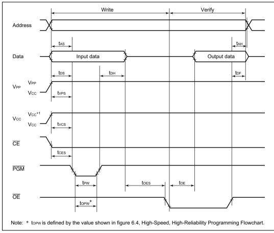
Figure 6.5 shows a PROM write/verify timing diagram.
