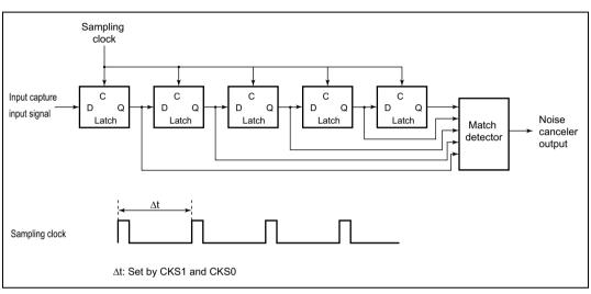
Figure 9.9 shows a block diagram of the noise canceler.
