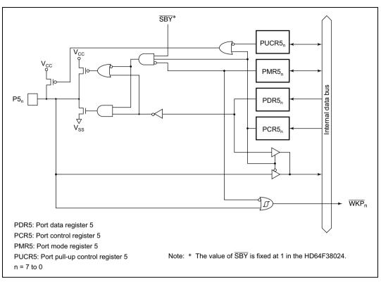
Figure C.4 Port 5 Block Diagram
