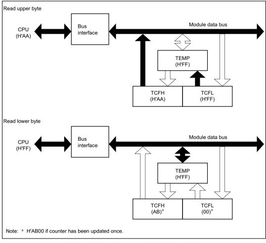
Figure 9.5 Read Access to TCF (TCF  $\rightarrow$  CPU)
