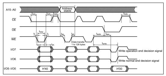
Figure 6.17 Auto-Program Mode Timing Waveforms
