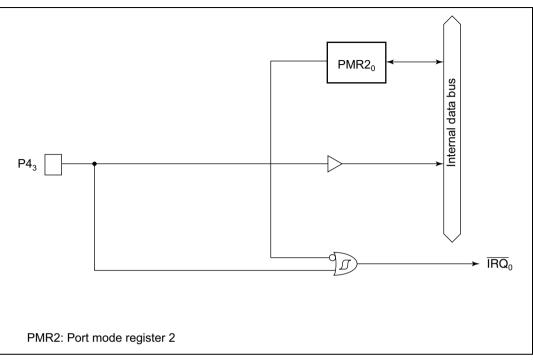
Figure C.3(a) Port 4 Block Diagram (Pin P4<sub>3</sub>)
