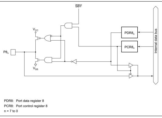
Figure C.7 Port 8 Block Diagram
