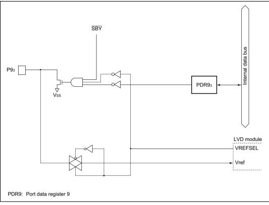
Figure C.8(c) Port 9 Block Diagram (Pins P9<sub>3</sub>, H8/38124 Group only)
