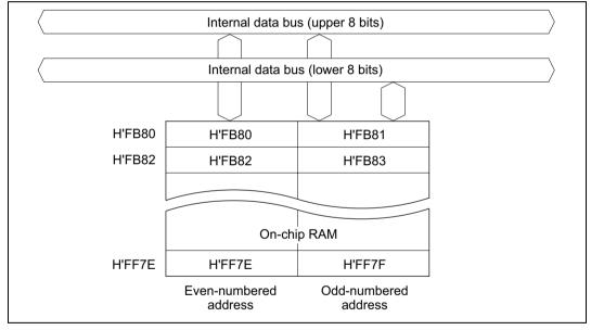
Figure 7.1 RAM Block Diagram (H8/38024)
