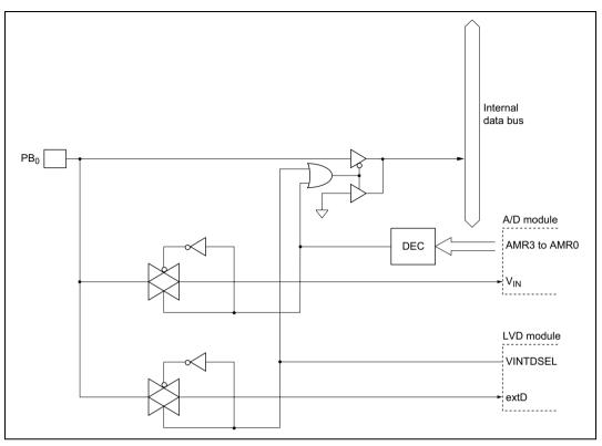
Figure C.10(b) Port B Block Diagram (Pin PB<sub>0</sub>, H8/38124 Group only)
