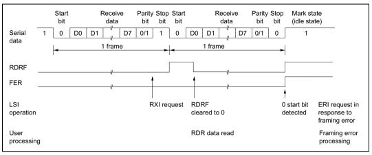
Figure 10.9 shows an example of the operation when receiving in asynchronous mode.
