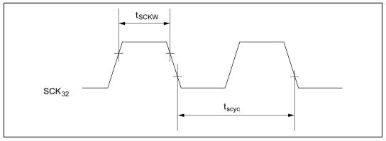
Figure 16.4 SCK3 Input Clock Timing
