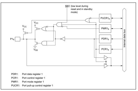
Figure C.1(b) Port 1 Block Diagram (Pin P1<sub>6</sub>, Products other than H8/38124 Group)
