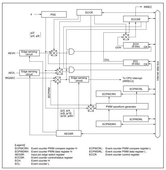
Figure 9.19 Block Diagram of Asynchronous Event Counter
