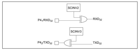
Figure 8.11 Input/Output Data Inversion Function
