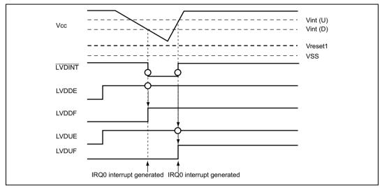
Figure 14.4 Operational Timing of LVDI Circuit
