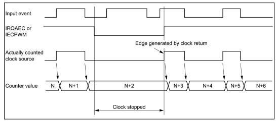
Figure 9.23 Example of Clock Control Operation
