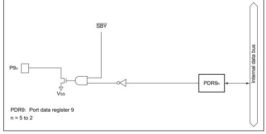
Figure C.8(b) Port 9 Block Diagram (Pins P95 to P92)
