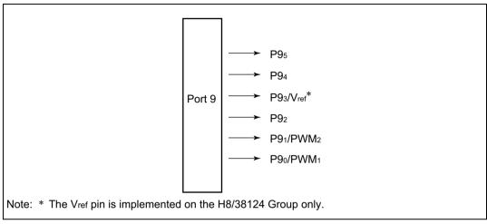
Figure 8.8 Port 9 Pin Configuration
