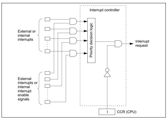
Figure 3.2 Block Diagram of Interrupt Controller
