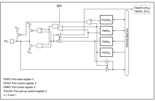
Figure C.2(d) Port 3 Block Diagram (Pins P3<sub>2</sub> and P3<sub>1</sub>)
