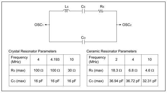
Figure 16.8 Resonator Equivalent Circuit (1)
