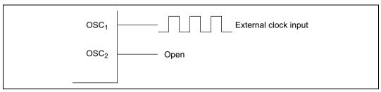
Figure 4.7 External Clock Input (Example)
