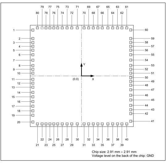
Figure 1.7 Bonding Pad Location Diagram of HCD64338024S, HCD64338023S, HCD64338022S, HCD64338021S, and HCD64338020S (Top View)
