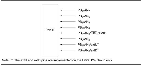
Figure 8.10 Port B Pin Configuration
