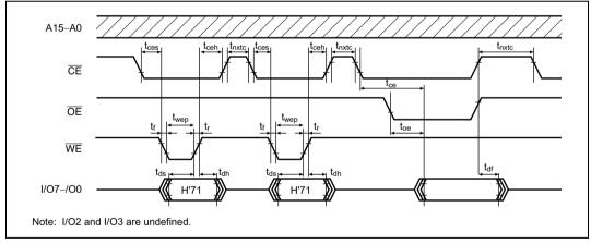
Figure 6.19 Status Read Mode Timing Waveforms
