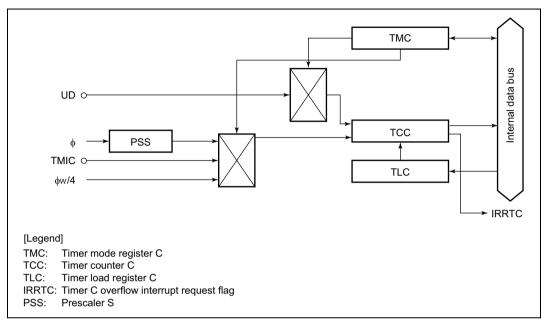
Figure 9.2 Block Diagram of Timer C
