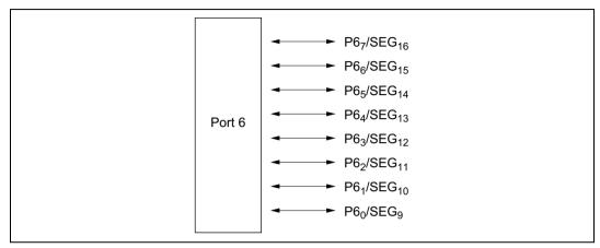
Figure 8.5 Port 6 Pin Configuration
