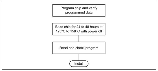
Figure 6.6 Recommended Screening Procedure
