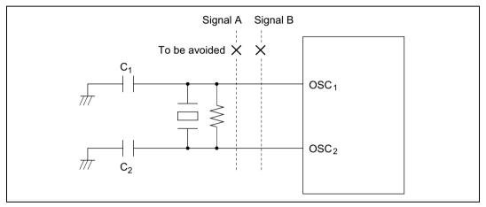
Figure 4.6 Board Design of Oscillator Circuit
