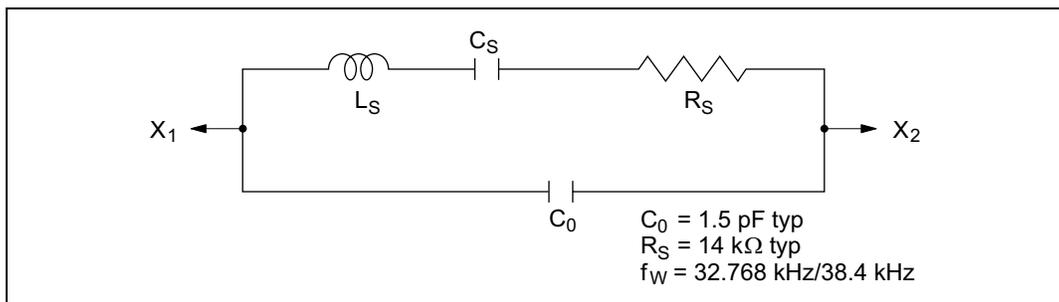
**Figure 4.9 Equivalent Circuit of 32.768 kHz/38.4 kHz Crystal Oscillator**
