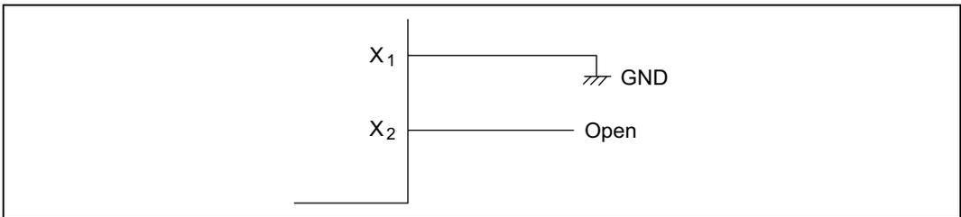
**Figure 4.10 Pin Connection when not Using Subclock**
