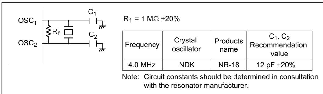
**Figure 4.3(2) Typical Connection to Crystal Oscillator
