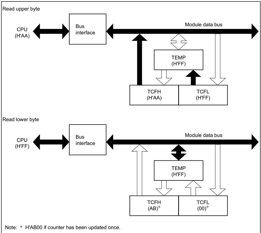
**Figure 9.5 Read Access to TCF (TCF → CPU)**
