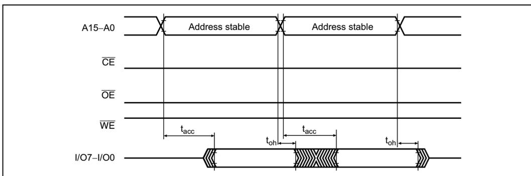
**Figure 6.15  $\overline{\text{CE}}$  and  $\overline{\text{OE}}$  Enable State Read Timing Waveforms**
