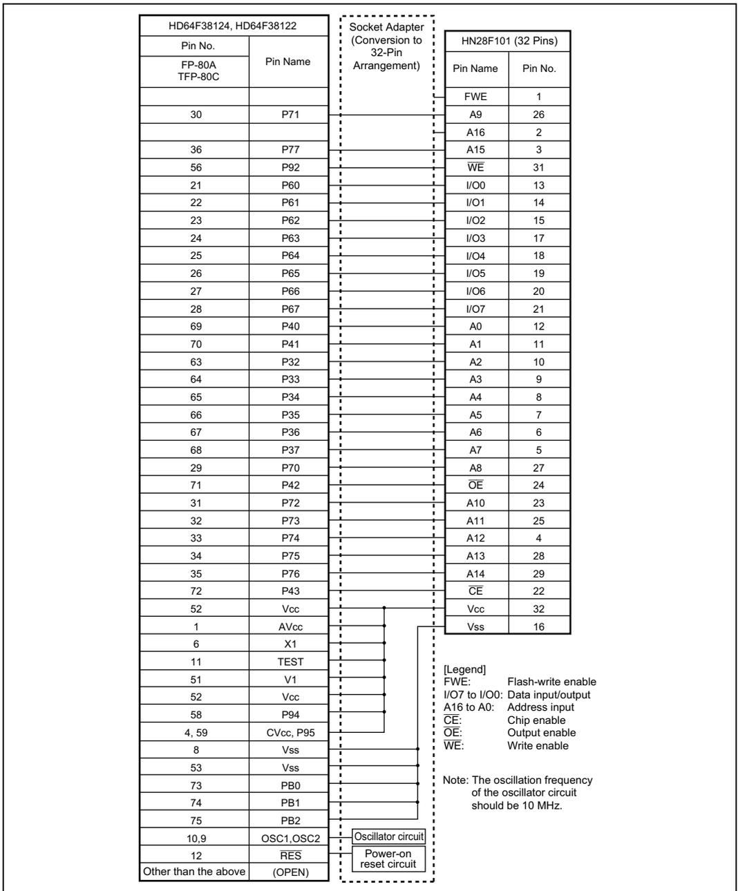
**Figure 6.12(2) Socket Adapter Pin Correspondence Diagram
