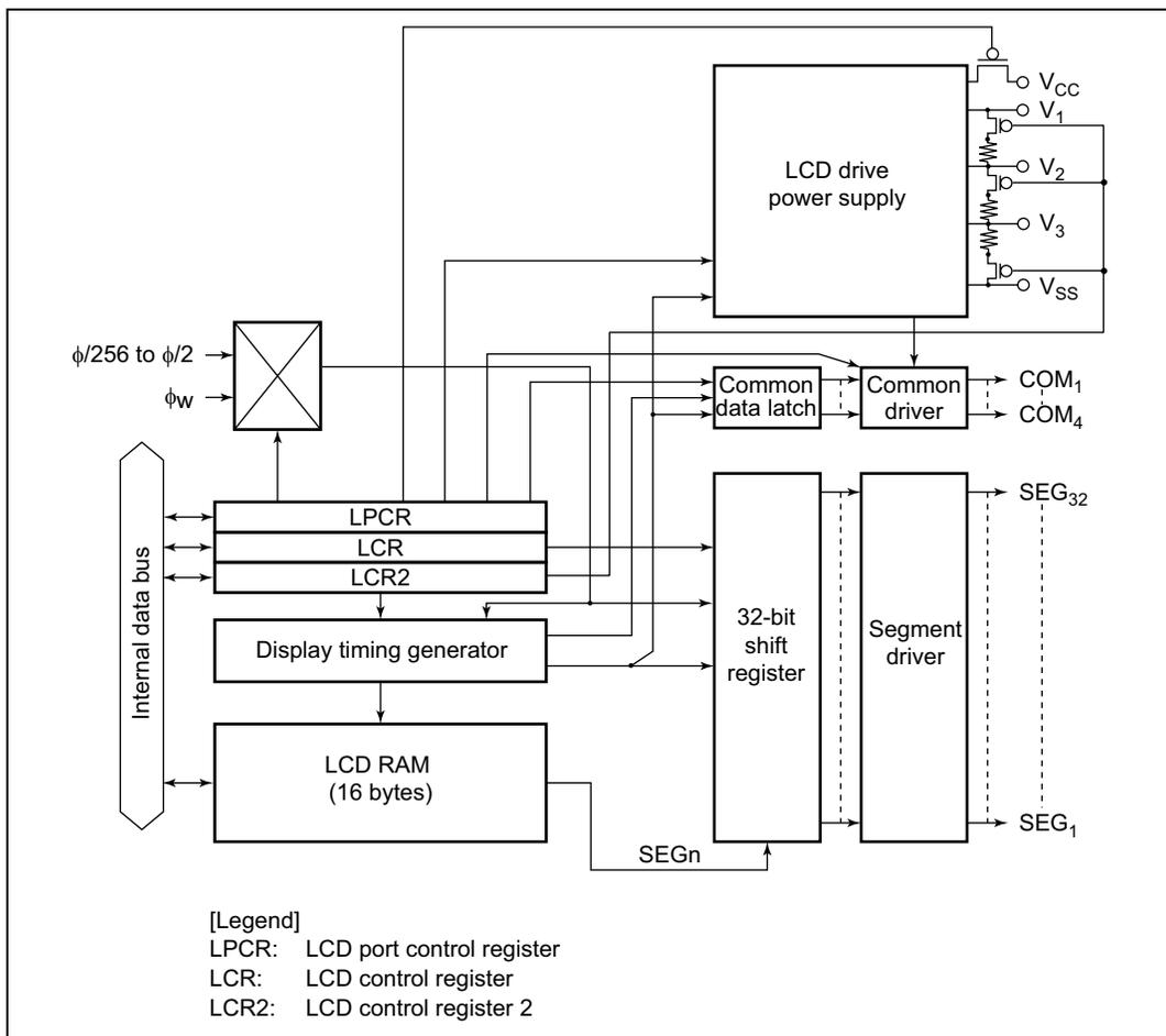
**Figure 13.1(2) Block Diagram of H8/38124 Group LCD Controller/Driver**
