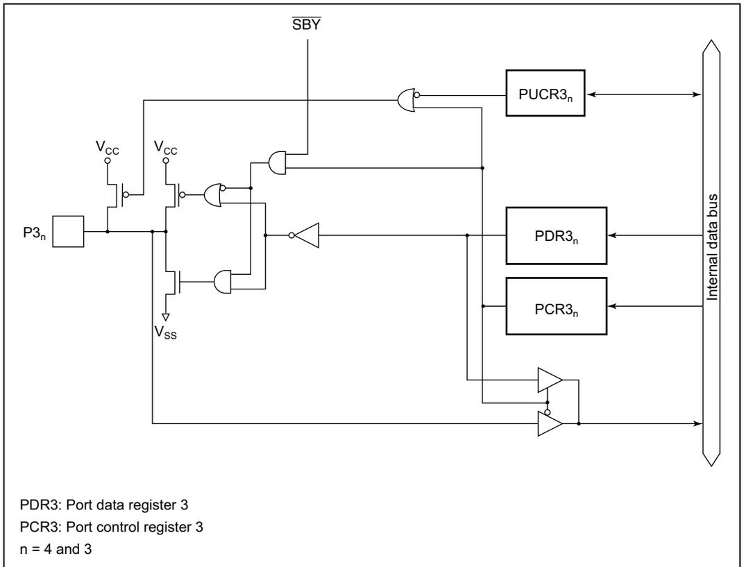
**Figure C.2(c) Port 3 Block Diagram (Pins P3<sub>4</sub> and P3<sub>3</sub>)**
