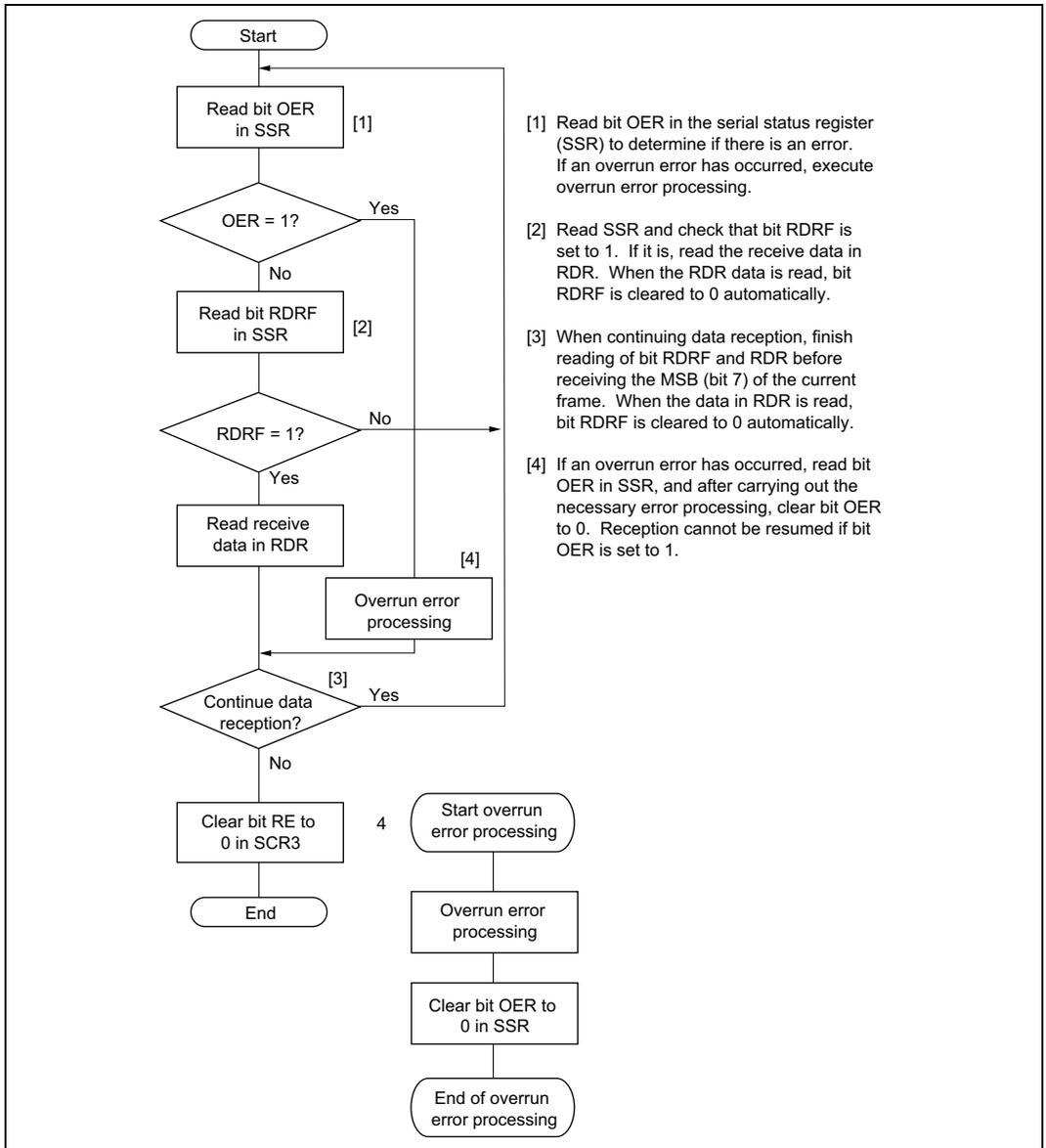
**Figure 10.13 Example of Data Reception Flowchart (Synchronous Mode)**
