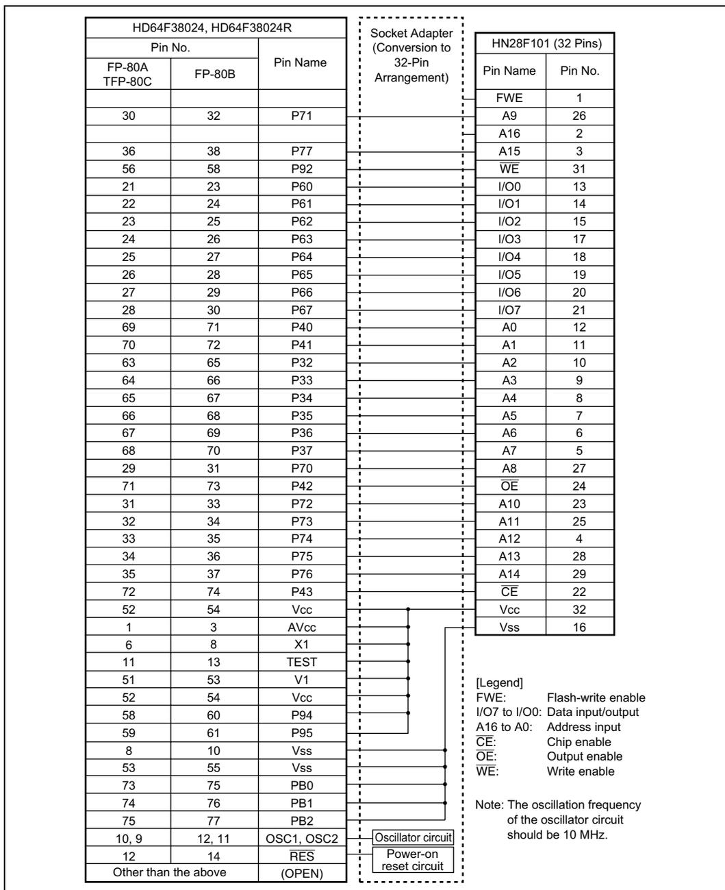
**Figure 6.12(1) Socket Adapter Pin Correspondence Diagram
