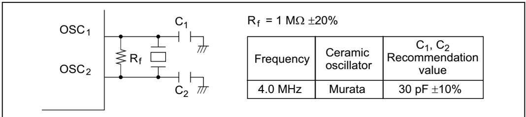
**Figure 4.5(1) Typical Connection to Ceramic Oscillator (H8/38024, H8/38024R Group)**
