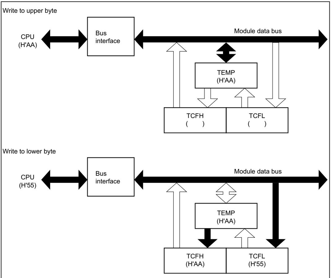
**Figure 9.4 Write Access to TCF (CPU → TCF)**
