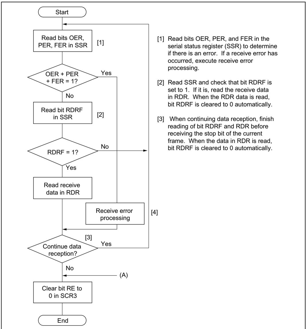
**Figure 10.8 Example of Data Reception Flowchart (Asynchronous Mode)**
