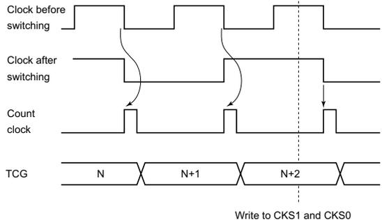
Note: \* The switchover is seen as a falling edge, and TCG is incremented.
