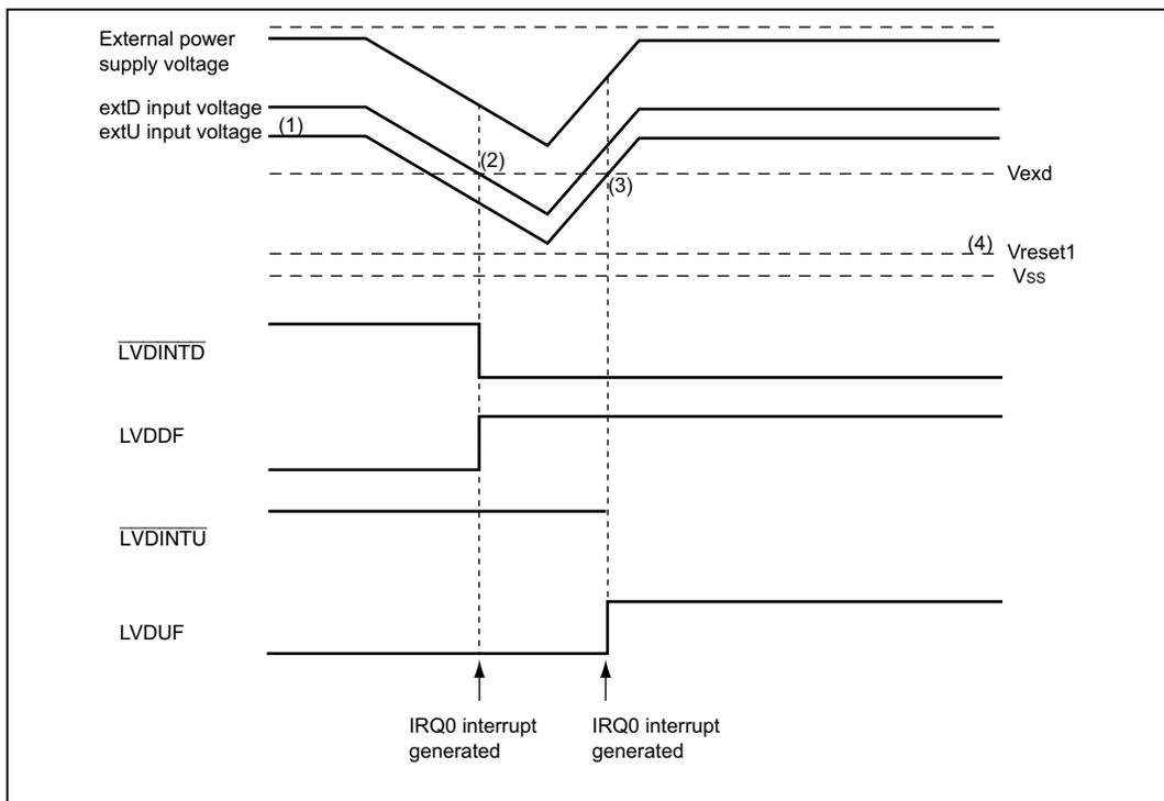
**Figure 14.5 Operational Timing of Low-Voltage Detection Interrupt Circuit
