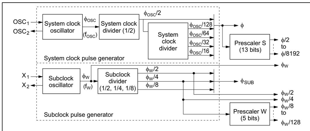
**Figure 4.1(1) Block Diagram of Clock Pulse Generators
