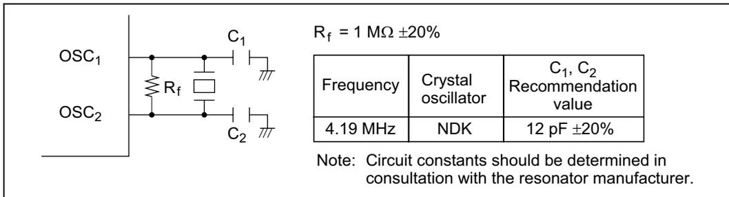
**Figure 4.3(1) Typical Connection to Crystal Oscillator
