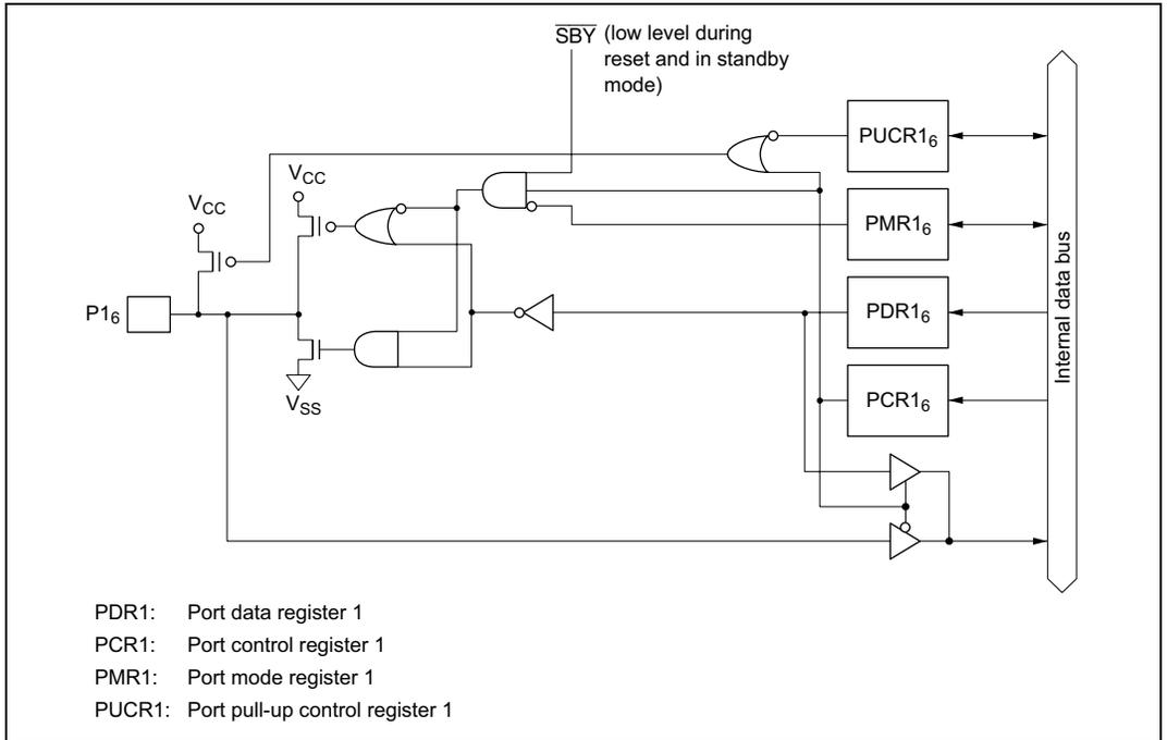
**Figure C.1(b) Port 1 Block Diagram (Pin P1<sub>6</sub>, Products other than H8/38124 Group)**
