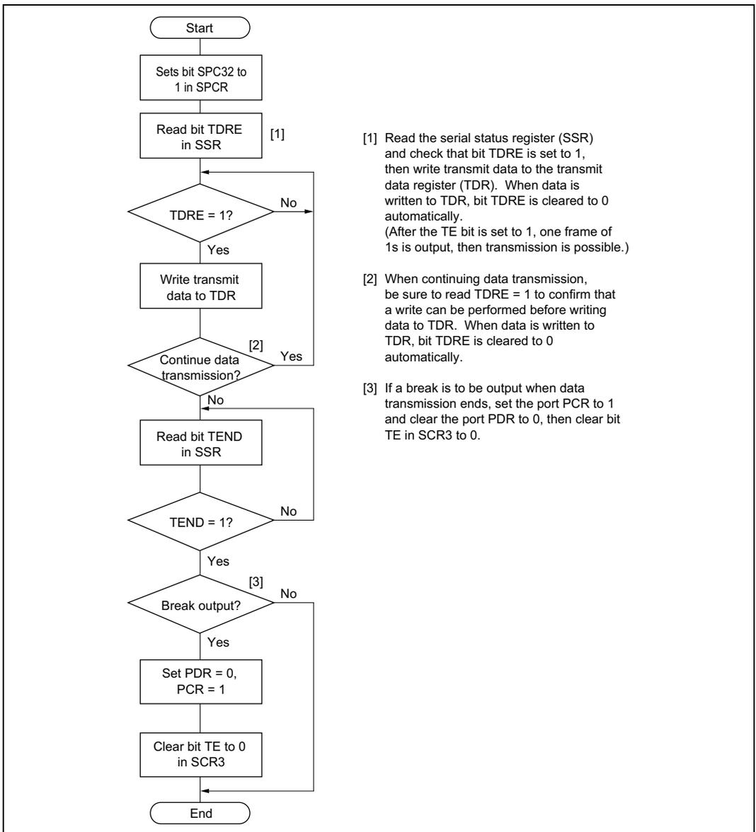
**Figure 10.6 Example of Data Transmission Flowchart (Asynchronous Mode)**
