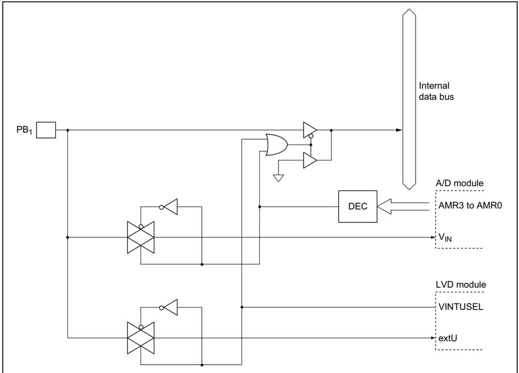
**Figure C.10(c) Port B Block Diagram (Pin PB<sub>1</sub>, H8/38124 Group only)**
