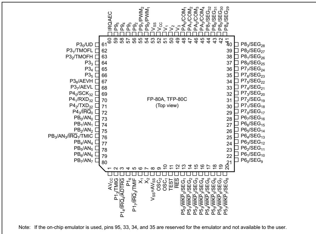
**Figure 1.2(1) Pin Arrangement (FP-80A, TFP-80C: Top View,
