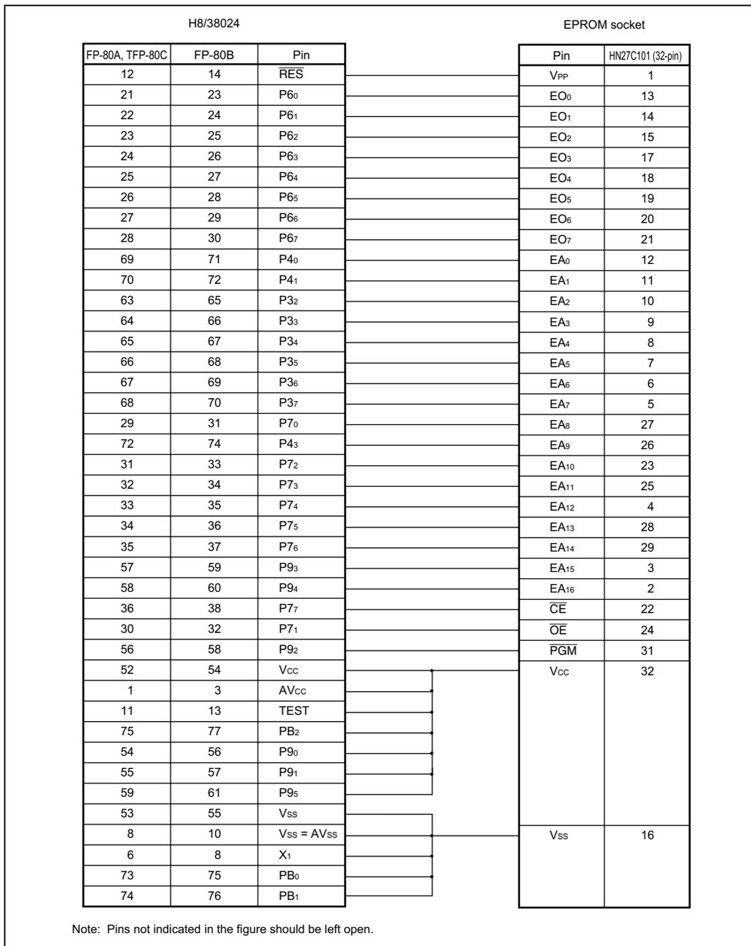
**Figure 6.2 Socket Adapter Pin Correspondence (with HN27C101)**
