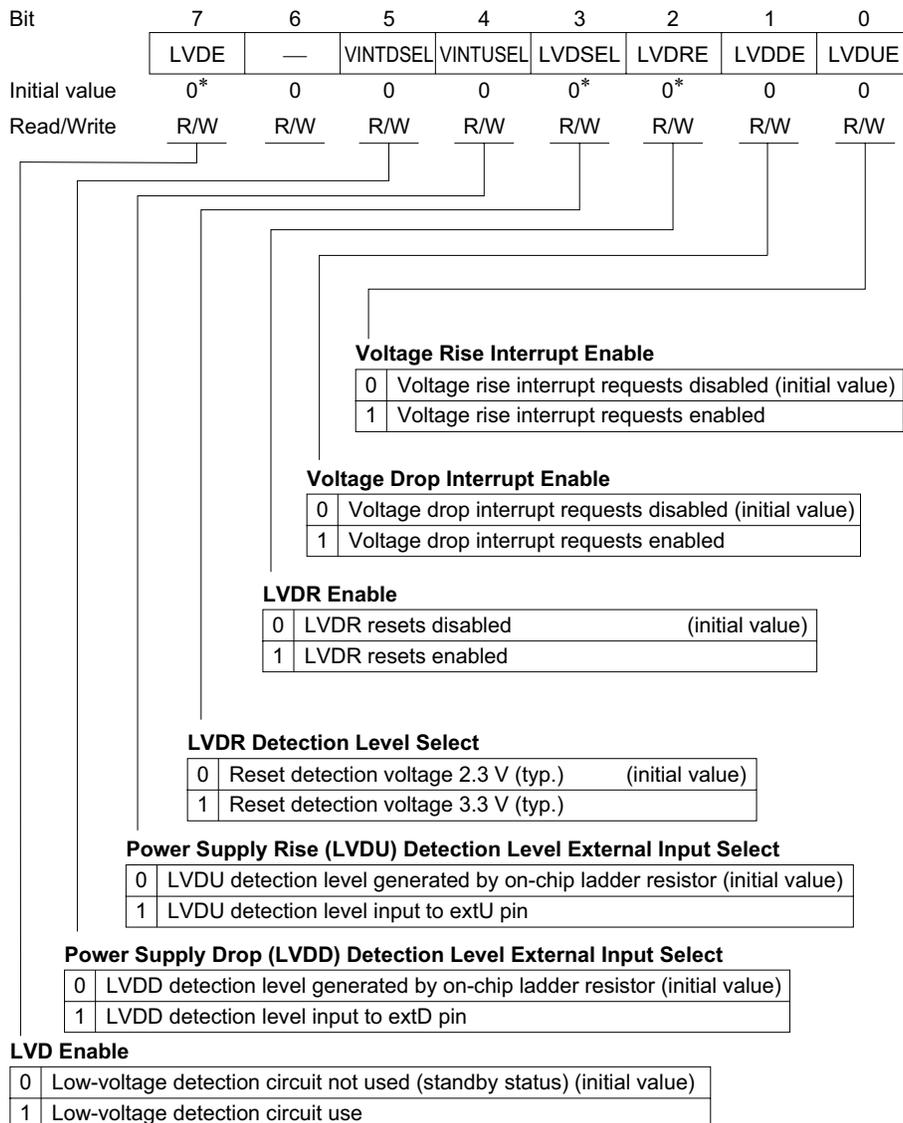
Note: \* These bits are not initialized by resets triggered by LVDR. They are initialized by power-on resets and watchdog timer resets.
