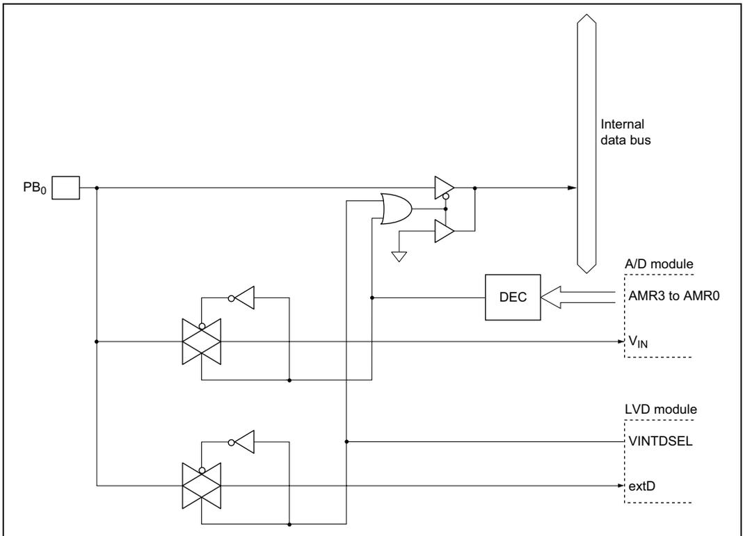
**Figure C.10(b) Port B Block Diagram (Pin PB<sub>0</sub>, H8/38124 Group only)**
