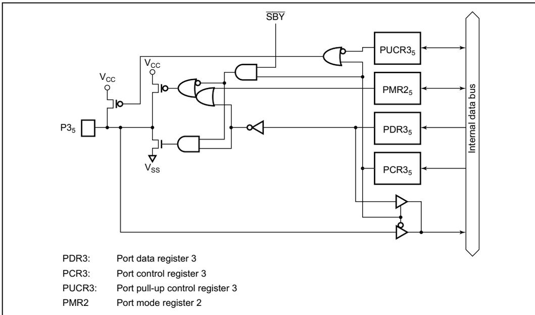
**Figure C.2(b) Port 3 Block Diagram (Pin P3<sub>5</sub>)**
