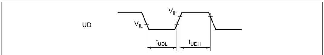
Figure 16.6 UD Pin Minimum Transition Width Timing
