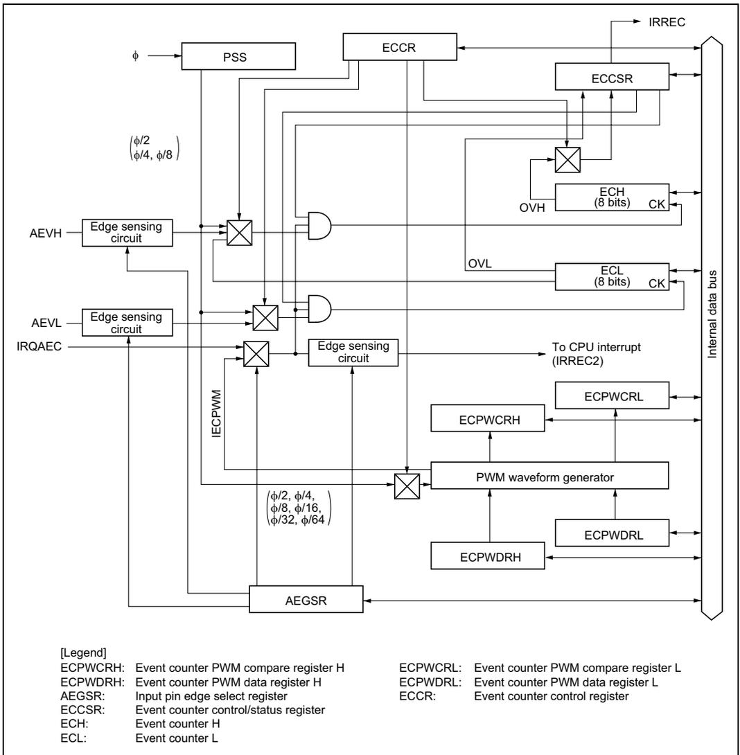
**Figure 9.19 Block Diagram of Asynchronous Event Counter**
