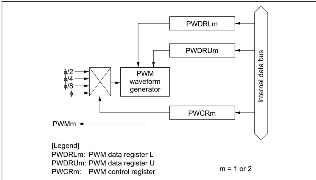
**Figure 11.1(1) Block Diagram of the 10-bit PWM
