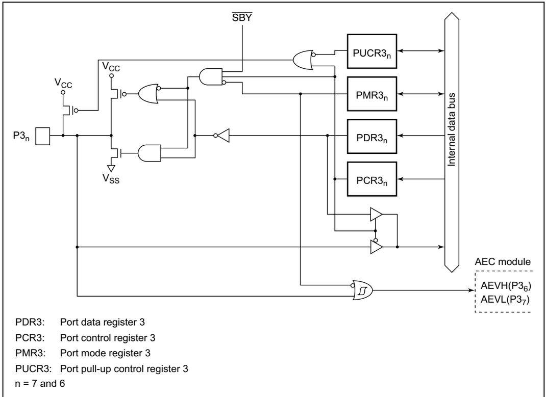
**Figure C.2(a) Port 3 Block Diagram (Pins P3<sub>7</sub> and P3<sub>6</sub>)**
