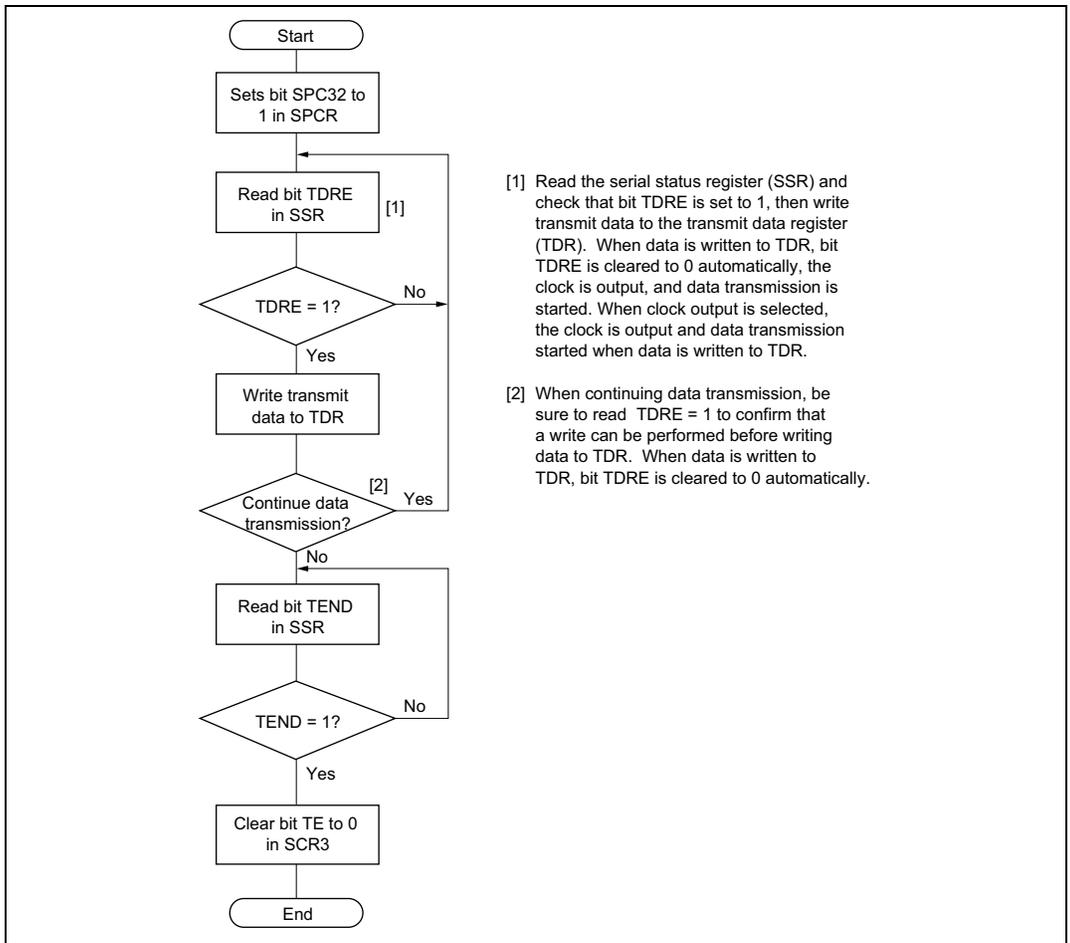
**Figure 10.11 Example of Data Transmission Flowchart (Synchronous Mode)**
