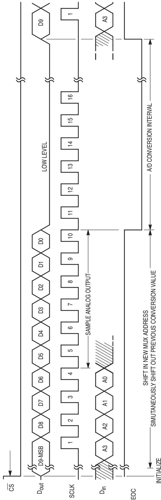
Figure 12. Timing for 16-Clock Transfer Not Using CS\* (Serial Transfer Interval Shorter than Conversion)
