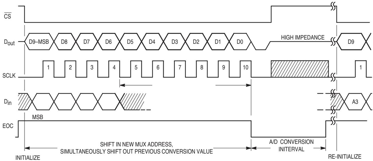
**Figure 9. Timing for 10-Clock Transfer Using  $\overline{CS}$**
