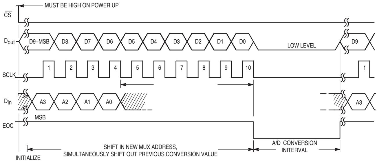
**Figure 10. Timing for 10-Clock Transfer Not Using  $\overline{CS}$**
