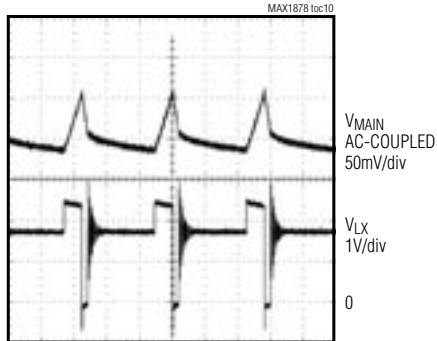
STEP-DOWN LIGHT-LOAD SWITCHING WAVEFORMS
