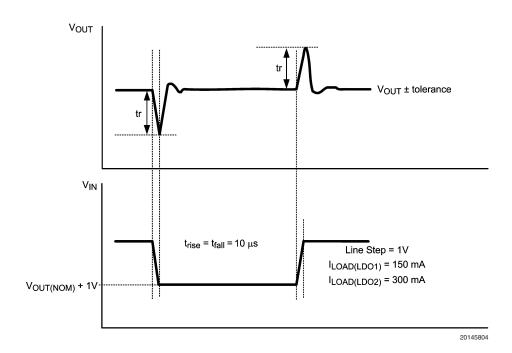
FIGURE 2. Line Transient Input Test Signal
