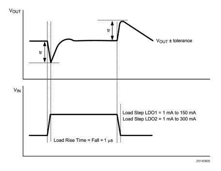
FIGURE 3. Load Transient Input Signal
