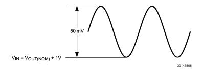
FIGURE 1. PSRR Input Signal
