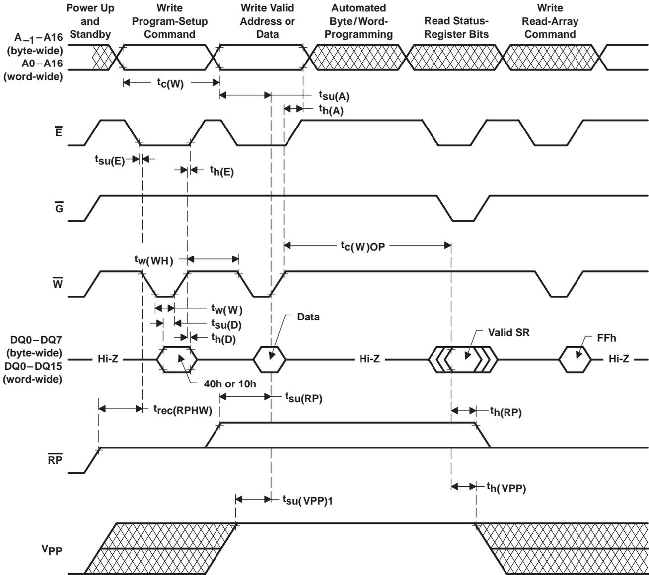
Figure 8. Write-Cycle Timing ( $\bar{W}$ -Controlled Write)
