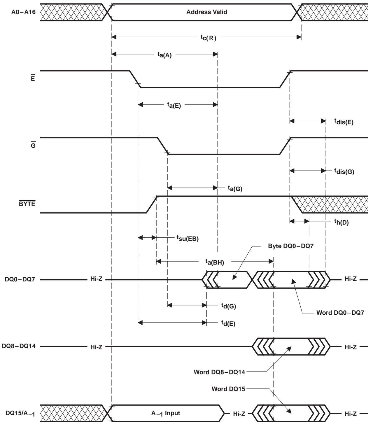
Figure 13.  $\overline{\text{BYTE}}$  Timing, Changing From Byte-Wide to Word-Wide Mode
