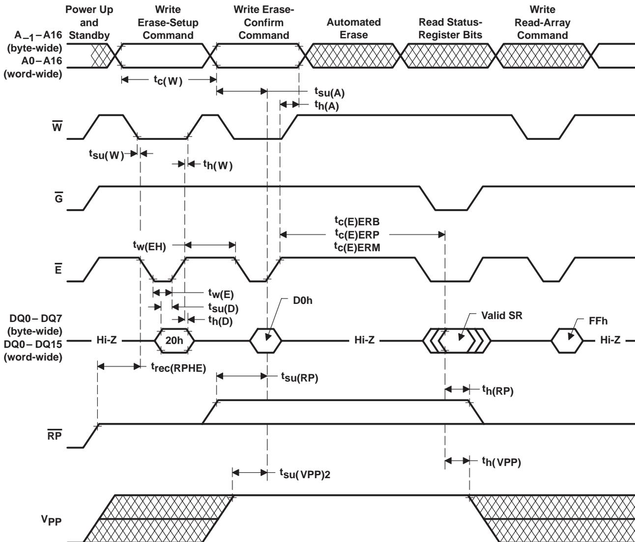
Figure 11. Erase-Cycle Timing ( $\bar{E}$ -Controlled Write)
