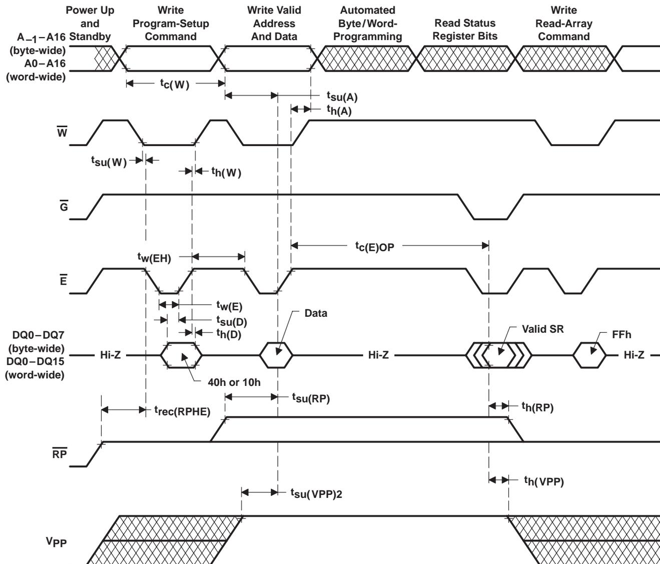
Figure 9. Write-Cycle Timing ( $\bar{E}$ -Controlled Write)
