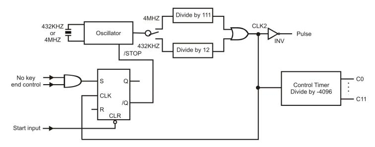
As you can see from the diagram above, the CLK1 (Oscillator Output) is divided by either 111 (for 4MHz) or by 12 (for 432KHz) depending on your mask option. CLK2 is used to control timer clocking. The frequency of CLK2 is 36KHz and its inverse is used to generate the output pulses in the subcarrier frequency. The duty factor may either be 25% or 33% depending on the mask option.
