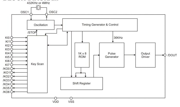
**Infrared Remote Control Transmitter IC**
