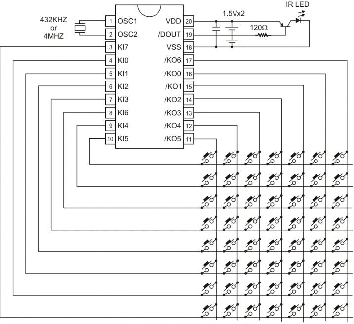
Note: External capacitors must be connected to generate the 432KHz Oscillation Frequency.
