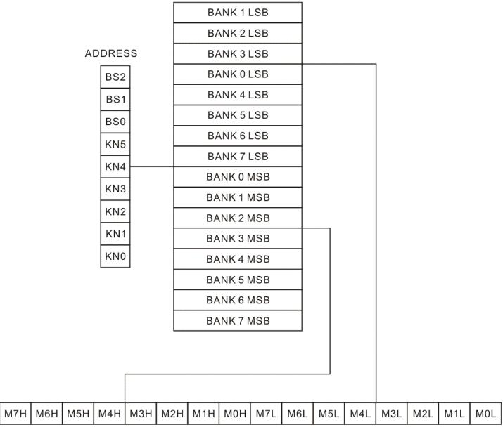
A bank is selected by using flip flops BS0 to BS2 which are the 3 highest address bits. In a single system, these bits are loaded from the 3 MSBs of the Scan Control when KI0 = "0". During Power-On, the bank select flip-flops will be in an arbitrary state.
