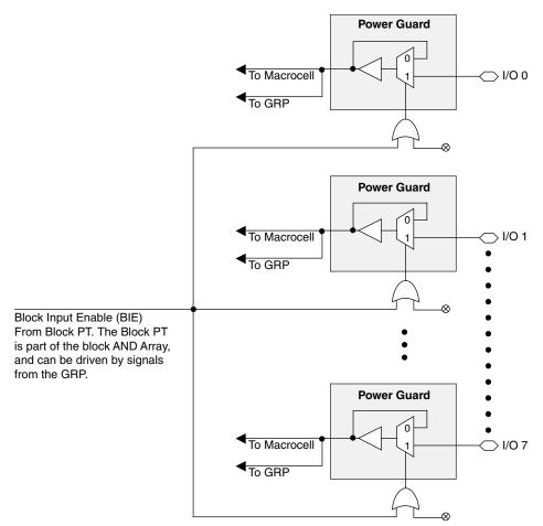
The number of BIE inputs, thus the number of Power Guard "Blocks" that can exist in a device, depends on the device size. Table 8 shows the number of BIE signals available in the ispMACH 4000ZE family. The number of I/Os available in each block is shown in the Ordering Information section of this data sheet.
