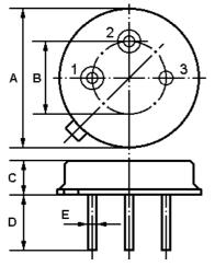
Pin Configuration Input / Output 1 2 Output / Input 3 Case Ground Dimension Data (unit: mm) 9.30±0.20 A 5.08±0.10 В С 3.40±0.20 D 3±0.20 / 5±0.20 Е 0.45±0.20
