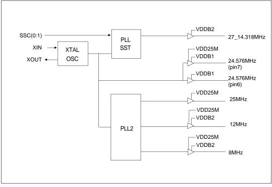
**Note:** In order to use VDD25M as power source for 8MHz (pin 13), 24.576MHz (pin 7), and 12MHz (pin 12), it is necessary to select this feature through the VDD\_SEL input (see Power Selection Table on p.1).
