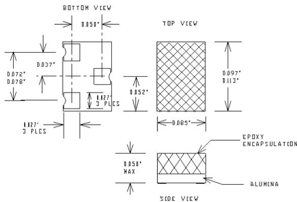
Packages are designed with wrap-around metallized castellations for superior assembly results.
