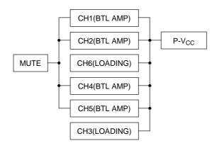
Note:  $\bullet$  Connect both S-V  $_{CC}$  and P-V  $_{CC}$  to the power supply system externally.
