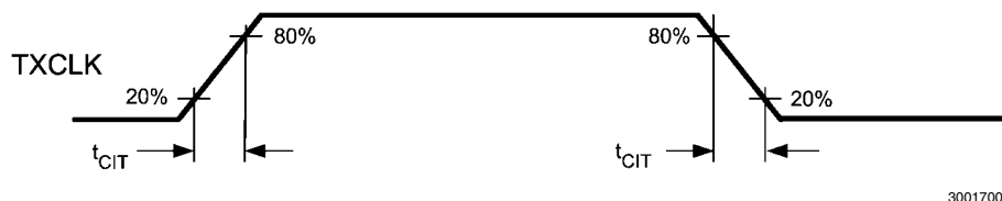
FIGURE 2. Transmit Clock Transition Times
