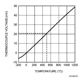
FIGURE 8. K-Type Thermocouple Response
