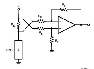
FIGURE 6. High-Side Current Sensing
