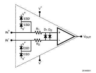
FIGURE 1. Protection Diodes between the Input Pins
