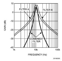
**FIGURE 5. Active Filter Curve**
