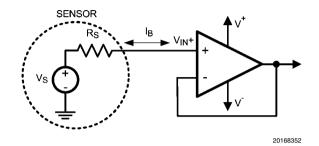
FIGURE 7. High Impedance Sensor Interface
