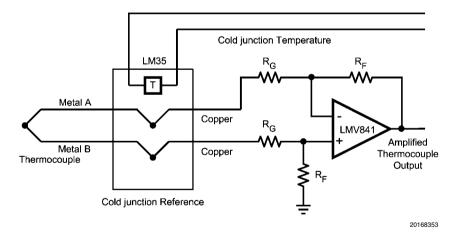
FIGURE 9. Thermocouple Amplifier
