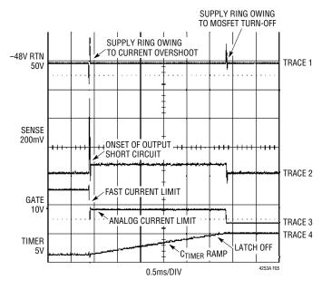
Figure 5. Output Short-Circuit Behavior of LTC4253A-ADJ
