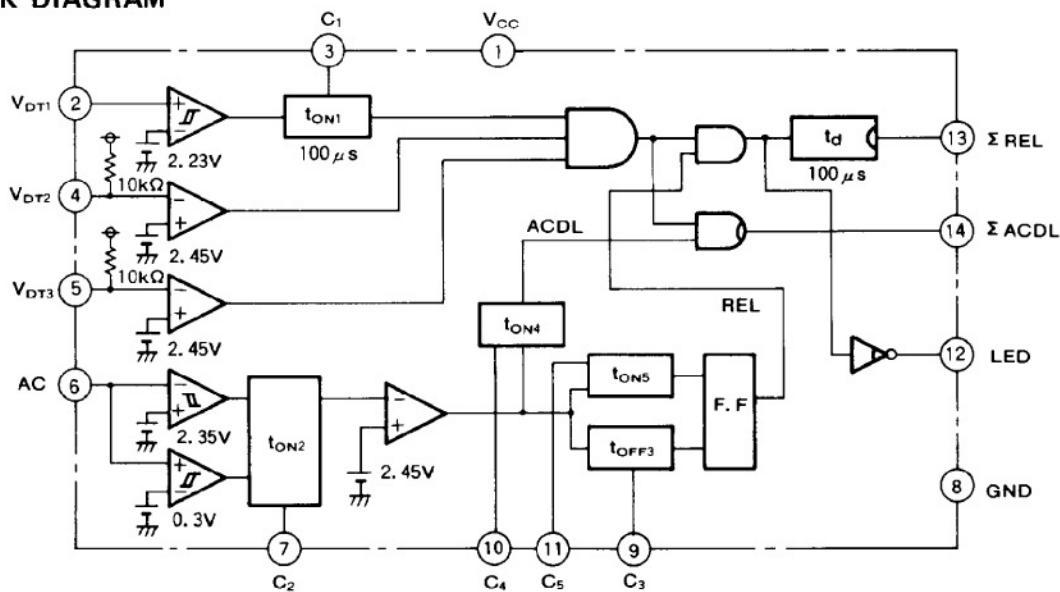
**AC-DC TOTAL SYSTEM RESET IC****ABSOLUTE MAXIMUM RATINGS** ( $T_a = 25^\circ\text{C}$ , unless otherwise noted)
