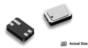
Vishay Thin film offers a four terminal hermetic leadless chip carrier package with precision matched pair elements. The network features tight ratio tolerance and close tracking over a 100  $\Omega$  to 100 k $\Omega$  resistance range. For custom schematics and values contact applications engineering.
