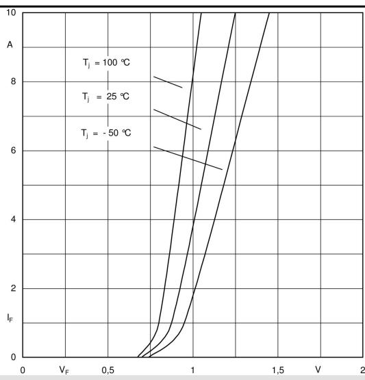
Fig. 1 Forward characteristics (typical values)
