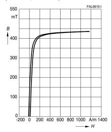
DC magnetic bias measured on ETD cores ( $\hat{B} \le 0.25$  mT, f = 10 kHz, T = 100 °C)
