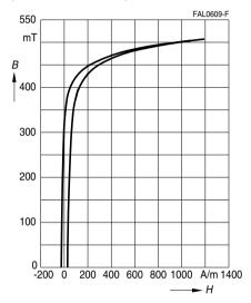
DC magnetic bias measured on ETD cores (B
