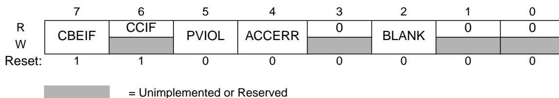
Figure 3-7 Flash Status Register (FSTAT)
