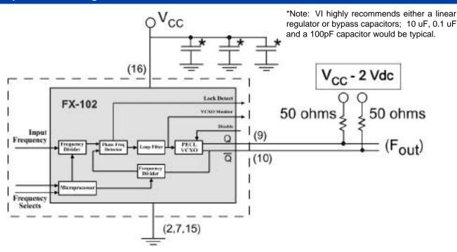
All components outside the dotted line box are user supplied components and/or connections. This is just one possible configuration of the FX-102. For additional information about your specific needs please contact our Factory.
