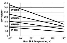
This graph shows the maximum wattage rating for each possible resistor of standard size corresponding to the heat sink temperature. It is assumed that all resistors are equally loaded.
