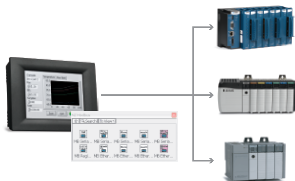
Figure 5. Modbus TCP/IP or ASCII Communication between a Touch Panel Computer and PLCs, RTU, or Modbus I/O
