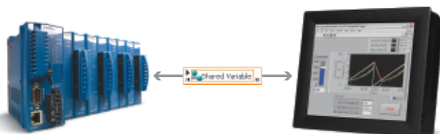
Figure 4. Shared-Variable Communication between NI PACs and a Touch Panel
