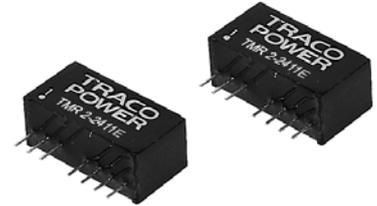
The TMR-2E series is a family of isolated 2W dc-dc converter modules with regulated output, featuring wide 2:1 input voltage ranges. The product comes in a compact SIP-8 plastic package with small footprint occupying only 2.0 cm<sup>2</sup> (0.3 square in.) of board space.
