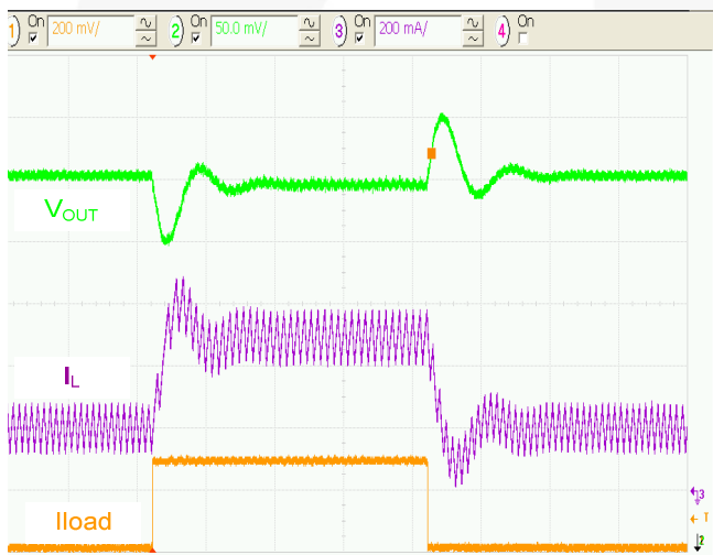
Figure 15. Load Transient 200 to 500mA, 3.6V IN , 5μs/div.
