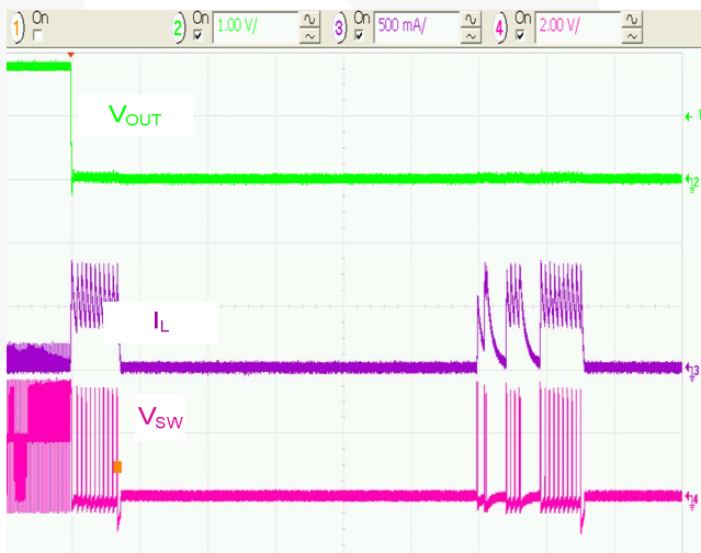
Figure 16. Metallic Short Applied at V OUT , 50μs/div.
