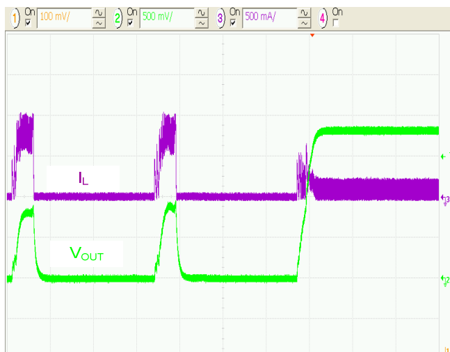
Figure 17. Overload Recovery to Light Load, 100μs/div.
