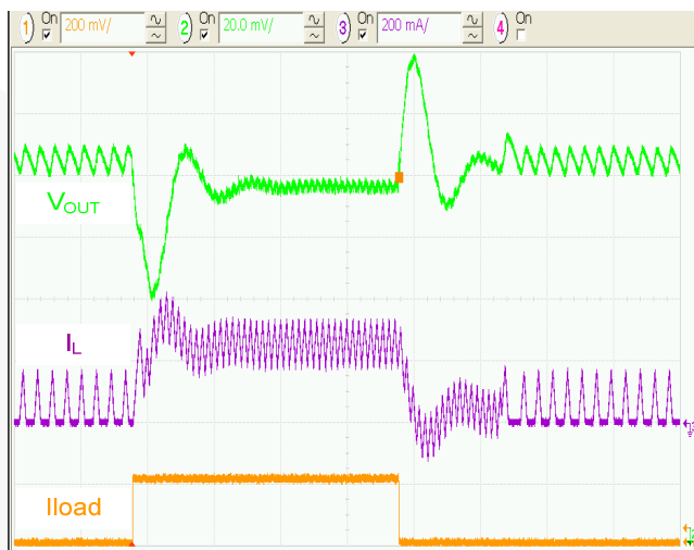
Figure 14. Load Transient 50 to 250mA, 3.6V IN , 5μs/div.
