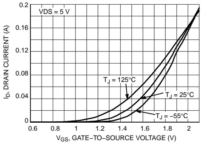
Figure 2. Transfer Characteristics
