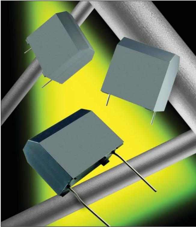
The FFB series uses a non-impregnated metallized polypropylene or polyester dielectric with the controlled self-healing process, specially treated to have a very high dielectric strength in operating conditions up to 105°C.
