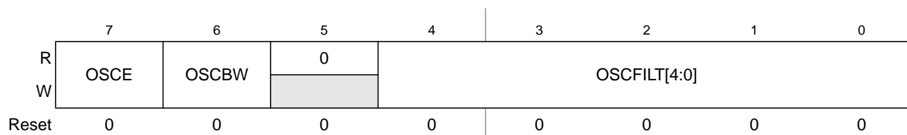
Figure 7-29. S12CPMU Oscillator Register (CPMUOSC)
