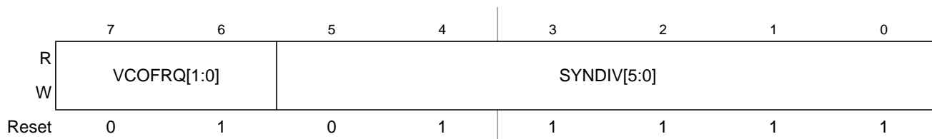
Figure 7-4. S12CPMU Synthesizer Register (CPMUSYNR)
