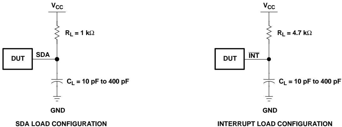
Figure 4. Load Circuits
