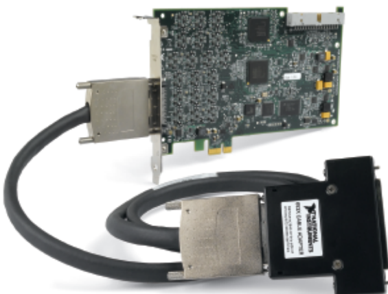
Figure 2. You can use NI 6535/36/37 devices with an NI 653x cable adapter to connect to existing NI 6533/34 applications.
