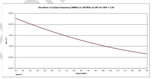
Note: Transition band is 30MHz to 34 MHz for VDD=2.5V at 25C. Deviation in this band is  $2.5\% \pm 4\%$ . Transition band is 30MHz to 39 MHz for VDD=3.3V at 25C. Deviation in this band is  $1.8\% \pm 30\%$ .
