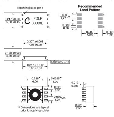
Dimensions are in  $\frac{\text{inches}}{\text{mm}}$
