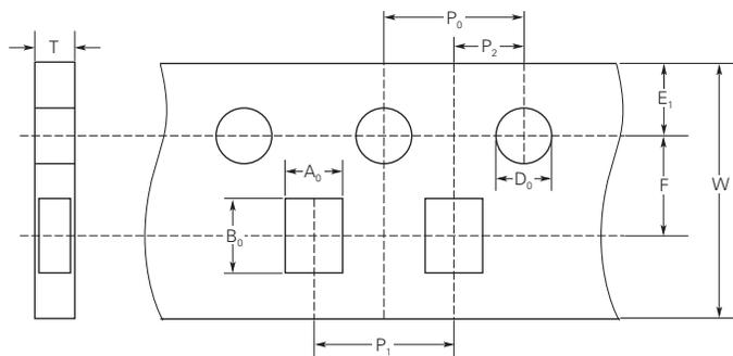
**Figure E12** EIA Referenced Reel Dimensions for ESD Devices
