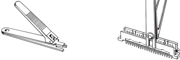
Cut the Coding Key on the Plug and insert the Coding Key in the Coding Key slots on the Socket to prevent improper insertion of the Plug into the Socket.
