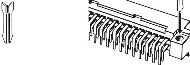
Fastening pins (XC5Z-0002) are used to keep the connector flush against the board during automated soldering.
