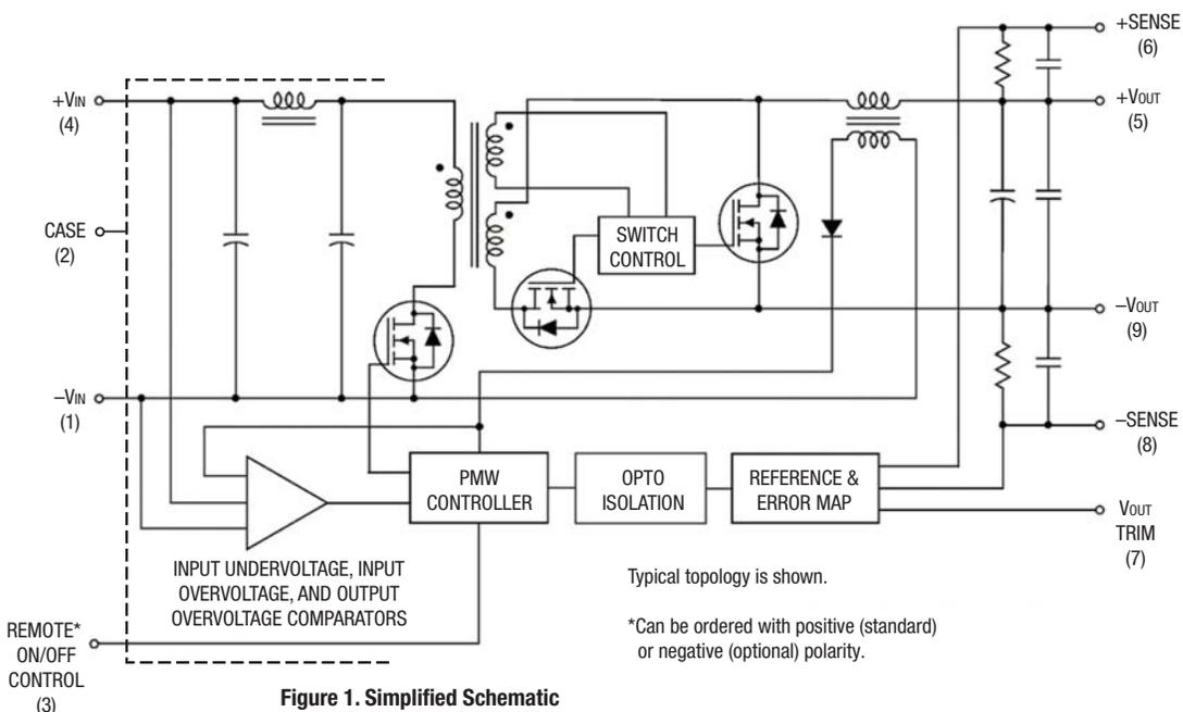
Figure 1. Simplified Schematic
