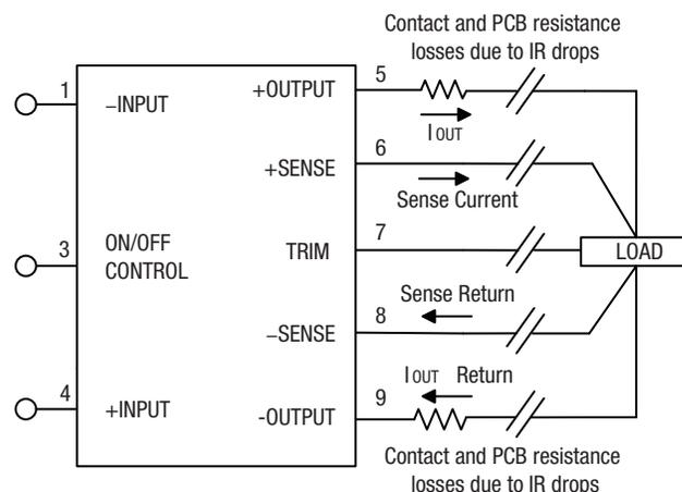
Figure 4. Remote Sense Circuit Configuration
