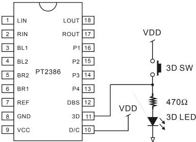
The 3D Switch toggles between activating and deactivating the 3D effect function. Under this mode, a 3D LED Display Indicator can be connected. When the 3D effect function is enabled, the LED is displayed. To make sure that the 3D effect function switching operation will work properly, the 3D pin trigger voltage value must not be less than 0.9VDD.
