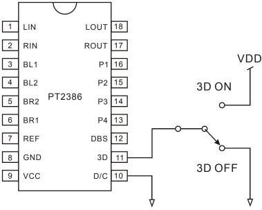
Under this condition, when the 3D pin is connected to VDD, the 3D effect function is activated. When the 3D Pin is connected to Ground, the 3D effect function is disabled. To make sure that the 3D effect function switching operation will work properly, the 3D pin trigger voltage value must not be less than 0.6VDD.
