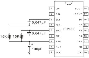
The bass booster level can be adjusted by changing the values of the external components (resistor/capacitor) connected to the Bass Booster Pins (BL1, BL2, BR1, BR2). If the value of the resistors connected to BR2, BL2 are decreased, the Bass Booster gain will increase. The typical resistor value is  $15K\Omega$ .
