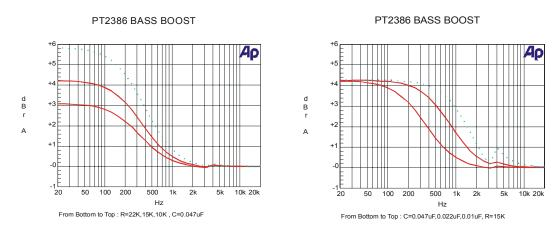
In order to avoid output clipping, it is recommended that the input signal be limited when the bass booster function is enabled. If the 3D function is switched ON and the bass booster function is not needed, then the bass booster pins -- BL1, BL2, BR1, BR2 must be "open".
