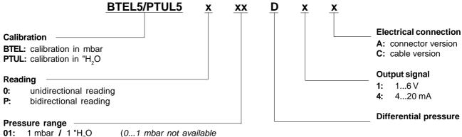
**01:** 1 mbar / 1 "H<sub>2</sub>O (0...1 mbar not available for output signal 1...6 V)
