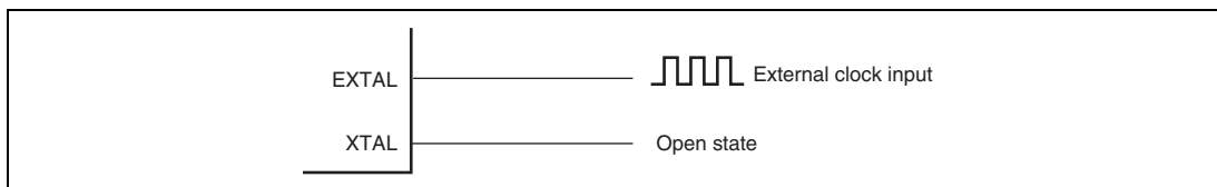
Figure 4.4 Example of External Clock Connection
