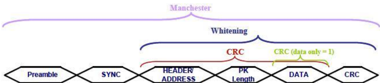
Figure 22. Operation of Data Whitening, Manchester Encoding, and CRC
